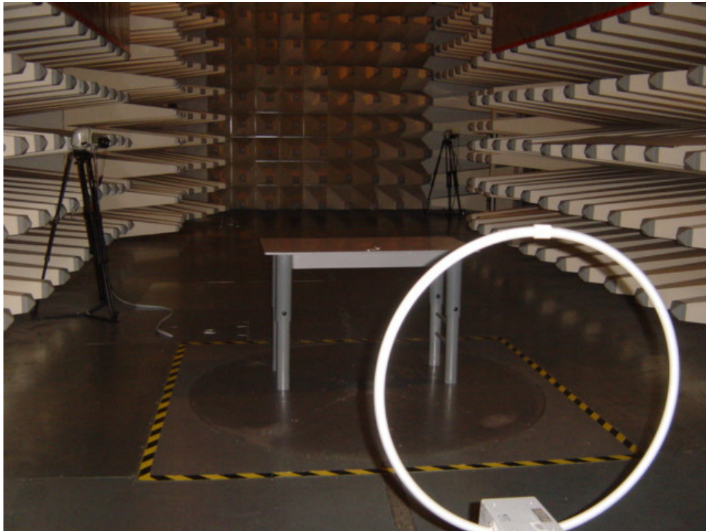
Set-up for Radiation Emission (Transceiver)
