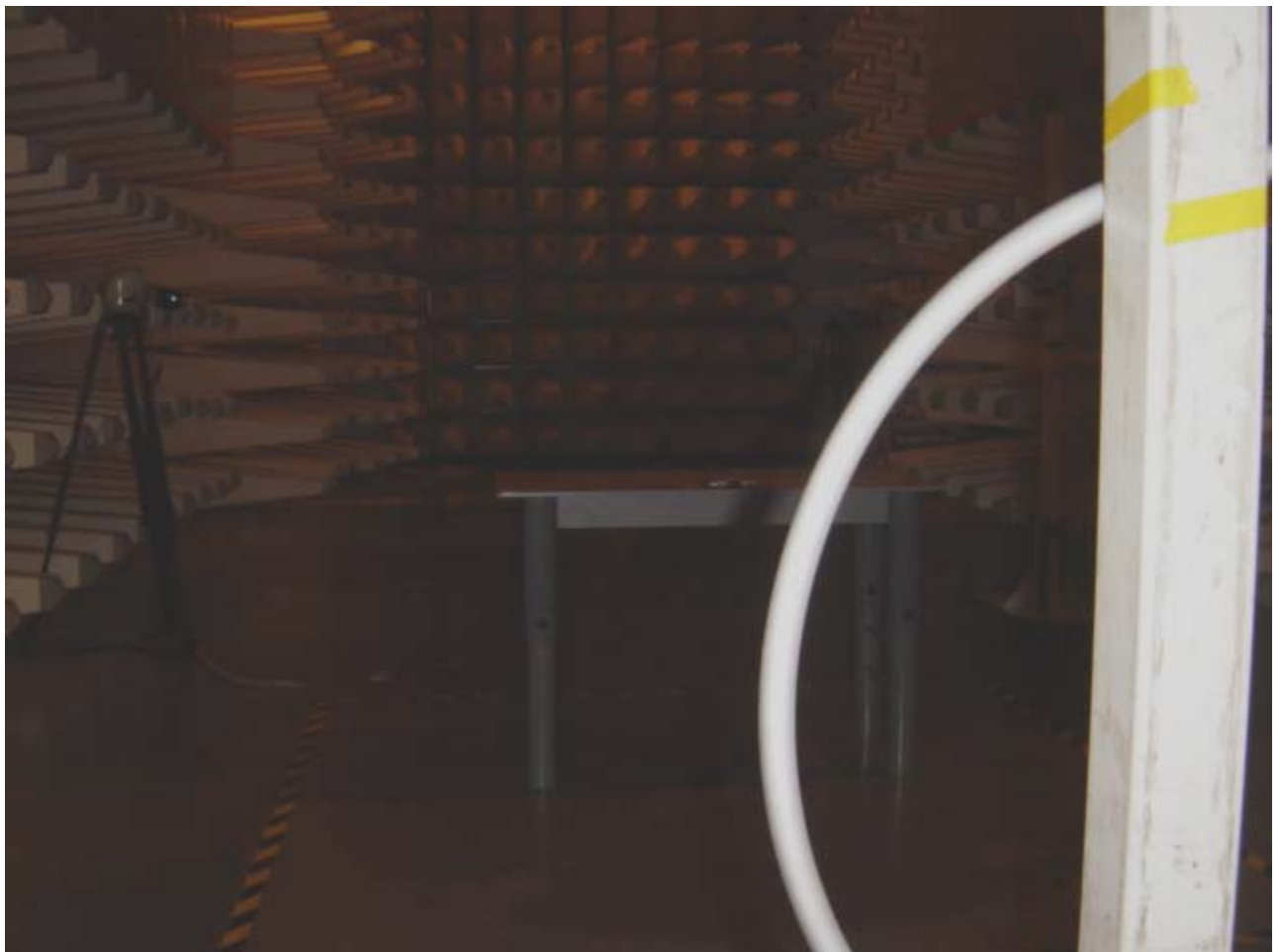
Set-up for Radiation Emission (Transceiver)
