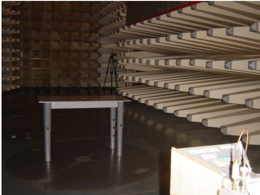
Set-up for Radiation Emission (Transceiver)
