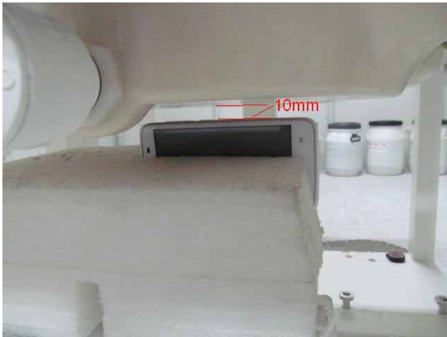
Body SAR Right Side 10mm for Wi-Fi
