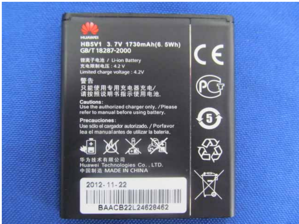
(7) EUT Photo (Battery #1)
