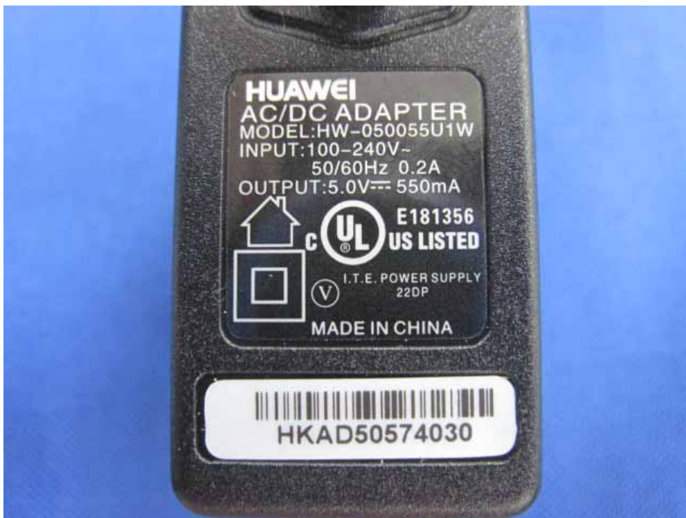
(12) EUT Photo (Adapter #1)
