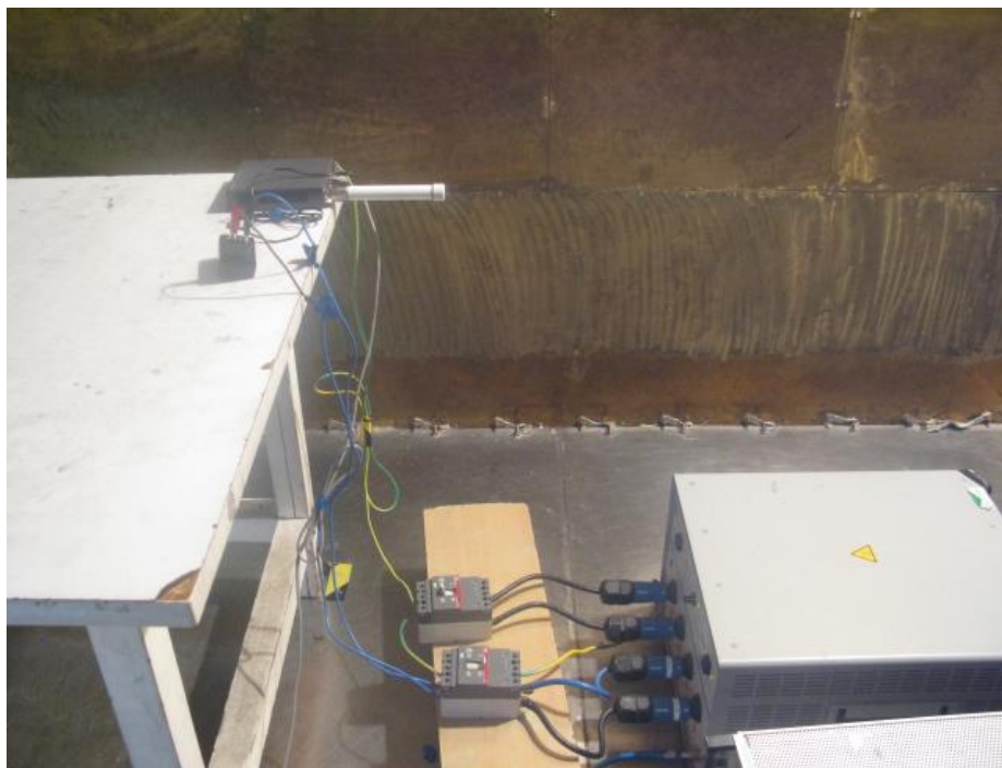
Conducted emissions of AC power port
