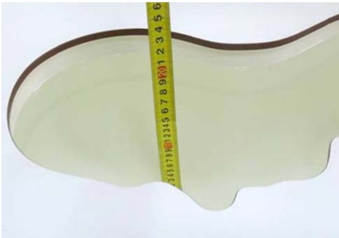
Picture 16: Liquid depth in the head Phantom (5300 MHz, 15.4cm depth)
