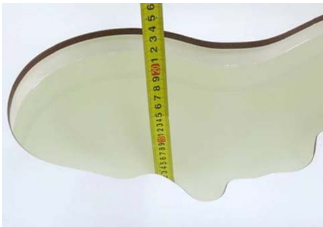
Picture 18: Liquid depth in the head Phantom (5600 MHz, 15.4cm depth)
