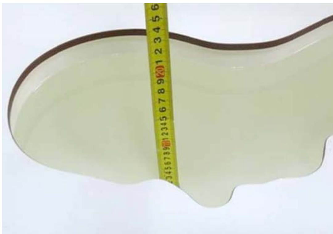
Picture 20: Liquid depth in the head Phantom (5800 MHz, 15.1cm depth)
