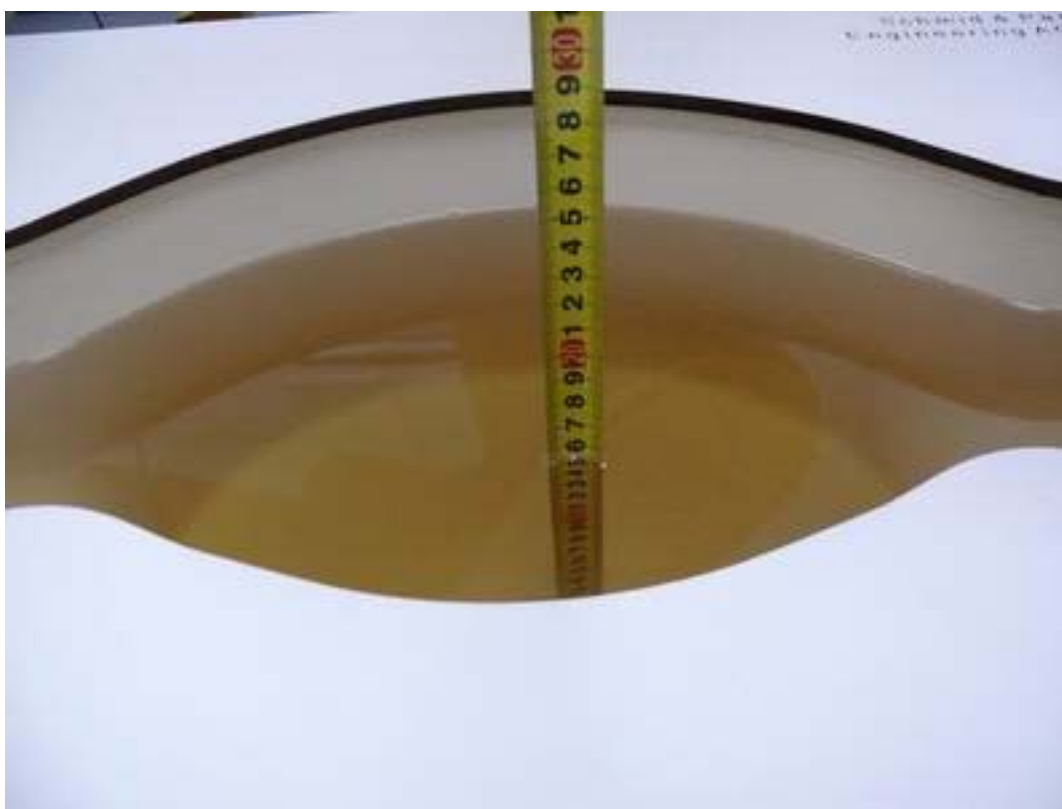
Picture 4: Liquid depth in the flat Phantom (750MHz, 15.4cm depth)
