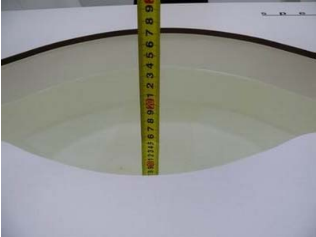
Picture 15: Liquid depth in the flat Phantom (5200 MHz, 15.3cm depth)
