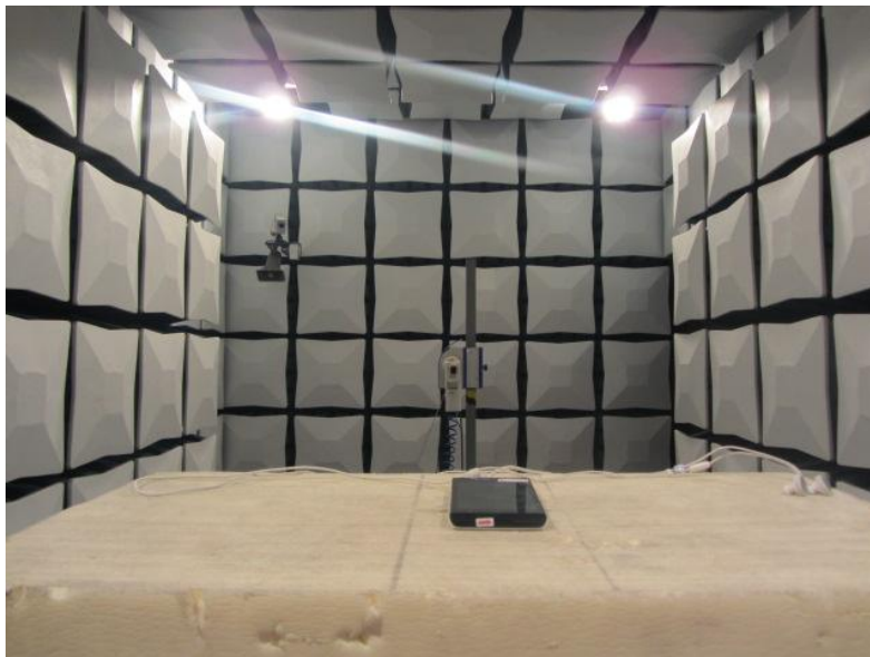
Radiated Spurious Emission (18GHz to26.5GHz)
