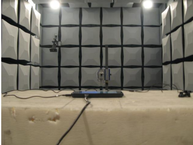
Radiated Spurious Emission (18GHz to26.5GHz)
