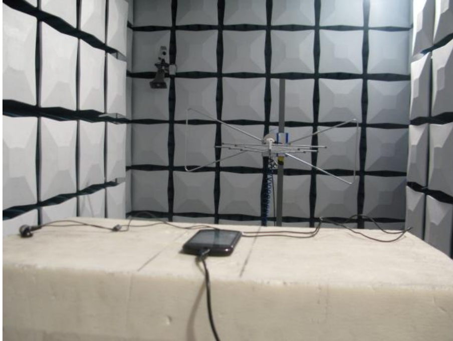
Field Strength of Spurious Emissions (below 3GHz)
