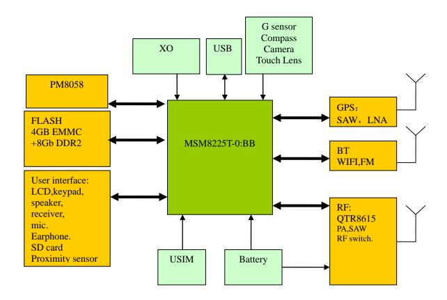
MSM8225T-0:Mobile Station Modem IC
