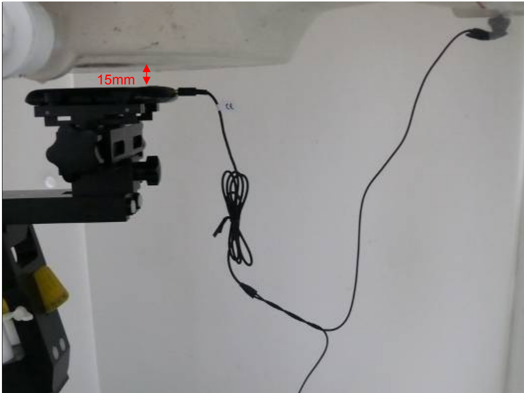
Picture 21: Back Side with earphone, the distance from handset to the bottom of the Phantom is 15mm
