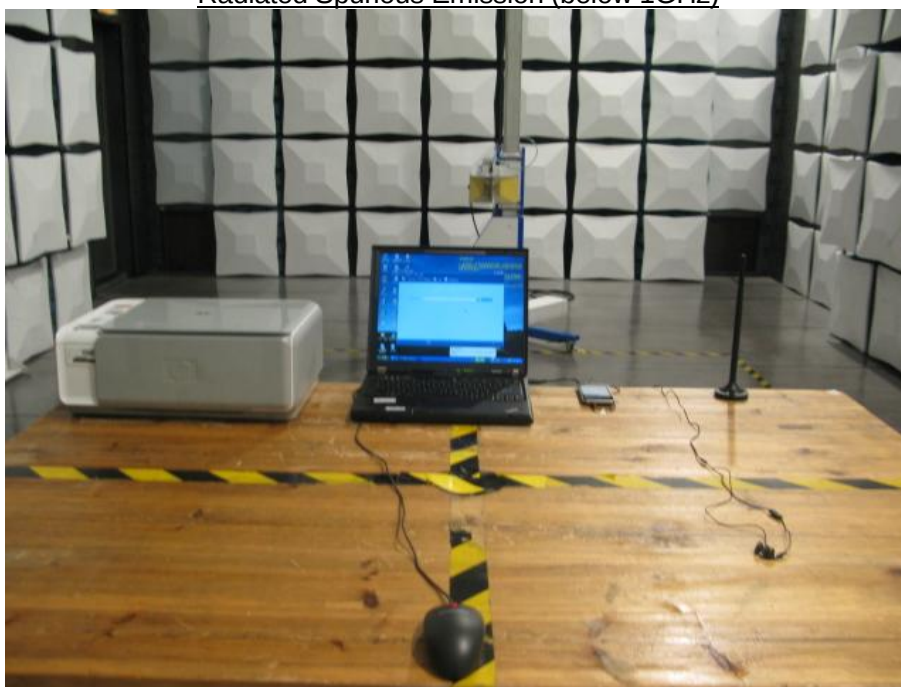
Radiated Spurious Emission (1GHz to 18GHz)
