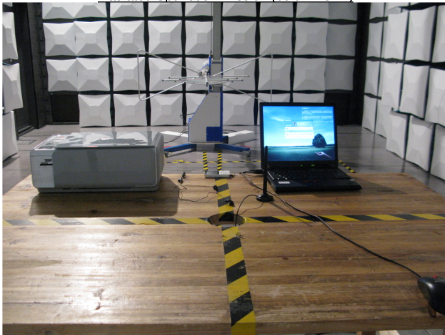
Radiated Spurious Emission (2GHz to 18GHz)
