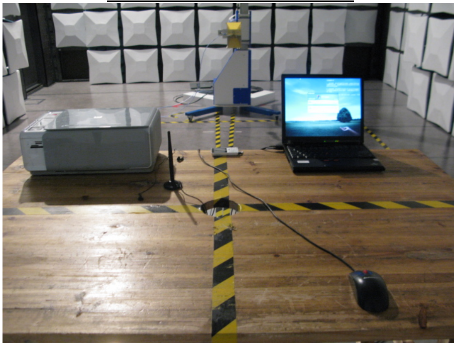
Radiated Disturbance (above 1GHz)
