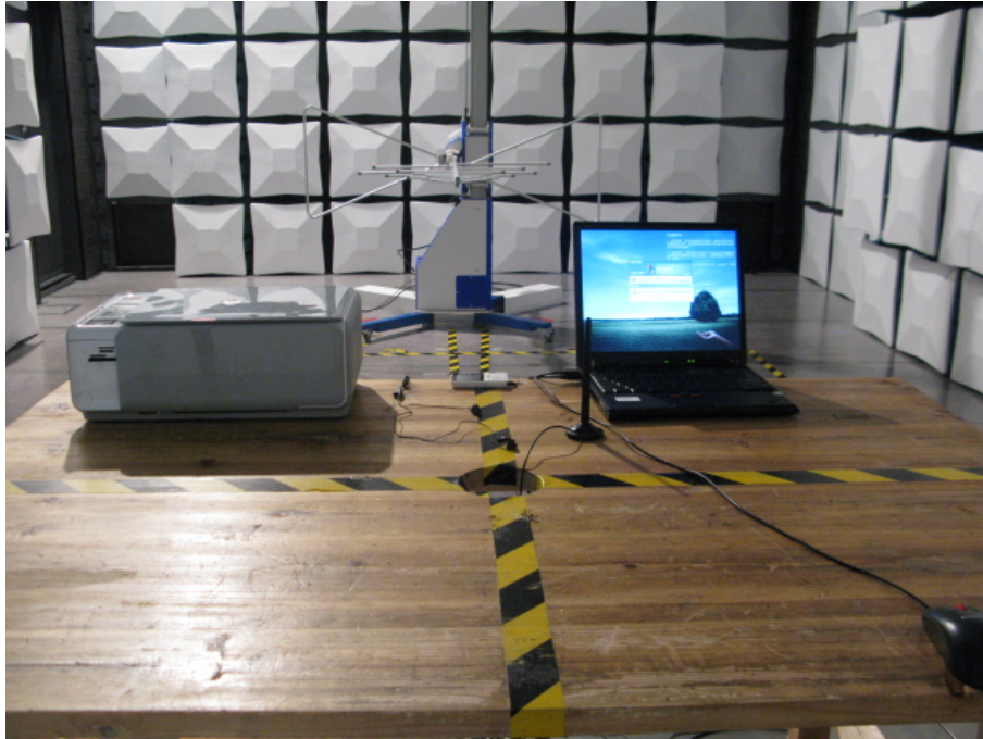
Radiated Disturbance (30MHz-1GHz)
