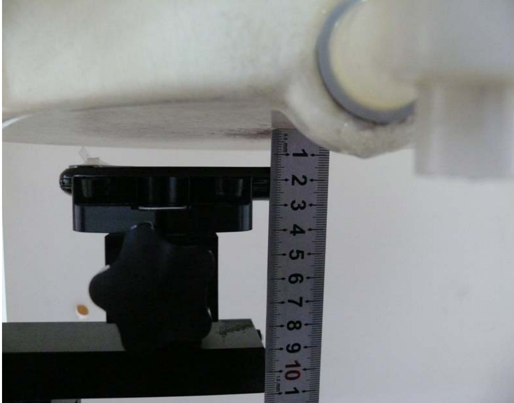
Picture 11: Body, The EUT display towards phantom, the distance from handset to the bottom of the Phantom is 15mm
