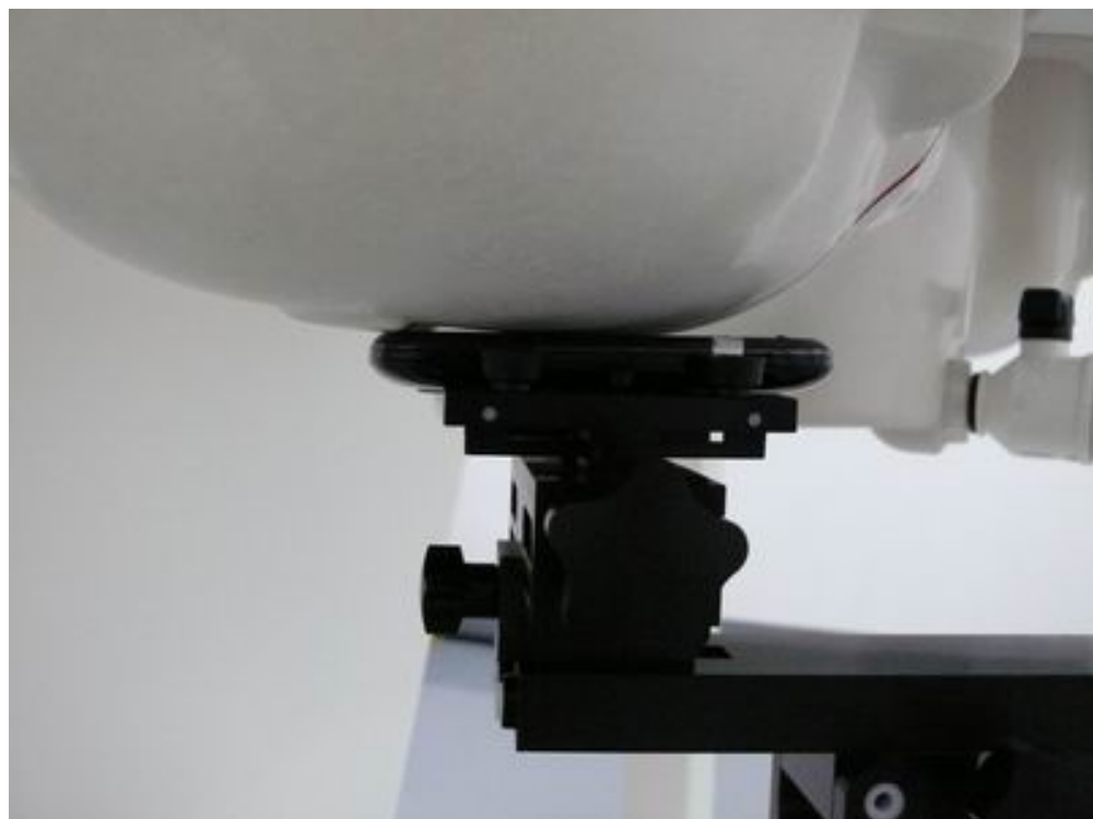
Picture 10: Right Hand Touch Cheek Position
