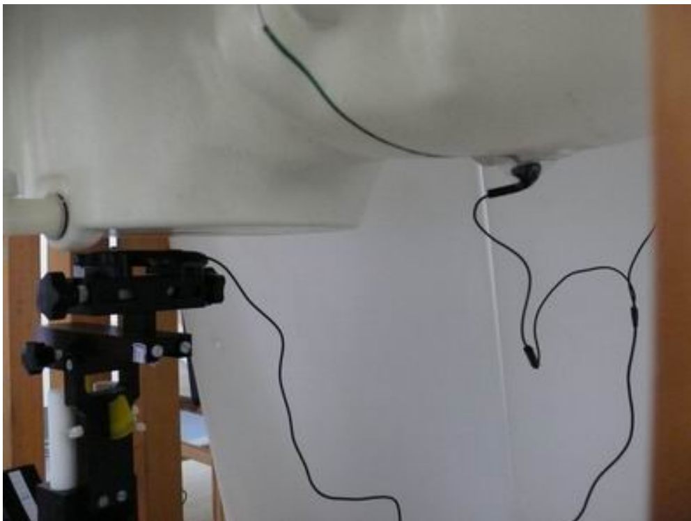
Picture 14: Body, The EUT display towards ground, the distance from handset to the bottom of the Phantom is 15mm
