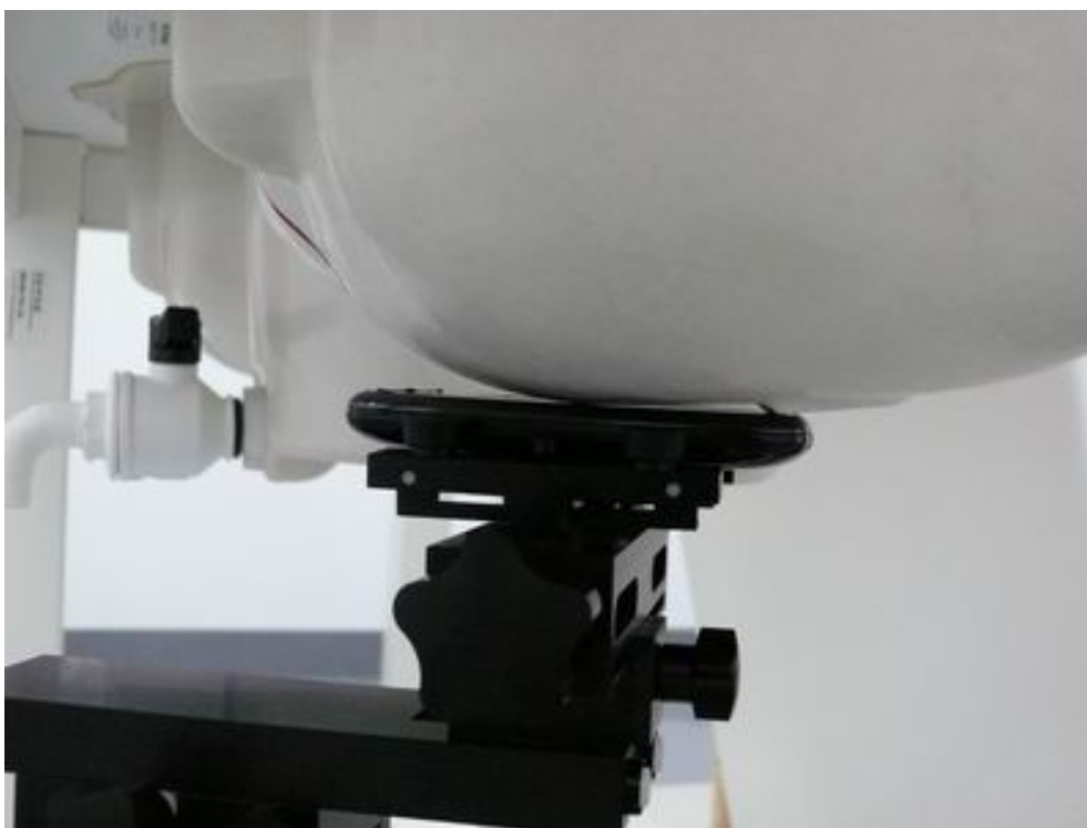
Picture 8: Left Hand Touch Cheek Position
