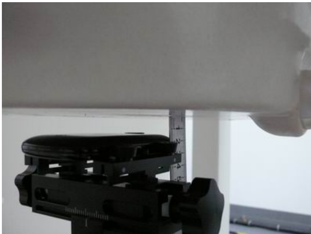
Picture 12: Body, The EUT display towards ground, the distance from handset to the bottom of the Phantom is 15mm
