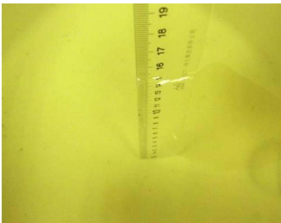
Picture 16-3: Liquid depth in the Flat Phantom (1900 MHz Head)
