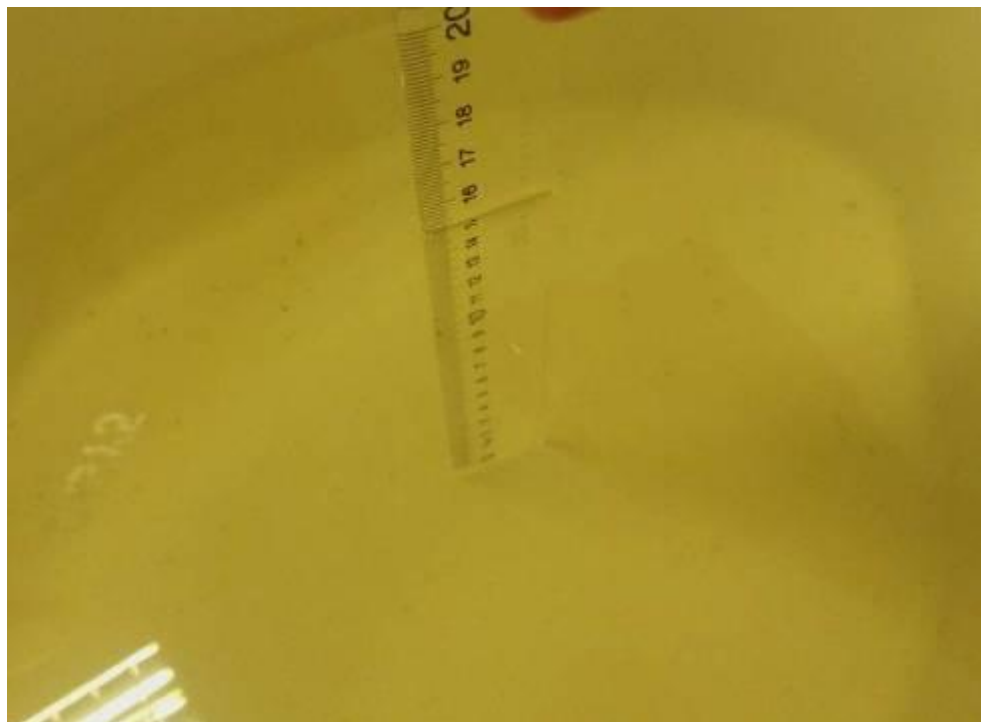
Picture 16-1: Liquid depth in the Flat Phantom (850 MHz Head)
