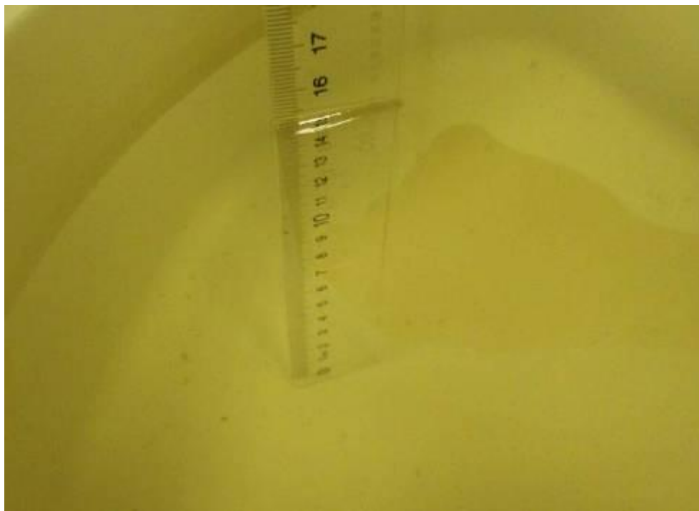
Picture 16-2: Liquid depth in the Flat Phantom (850 MHz Body)
