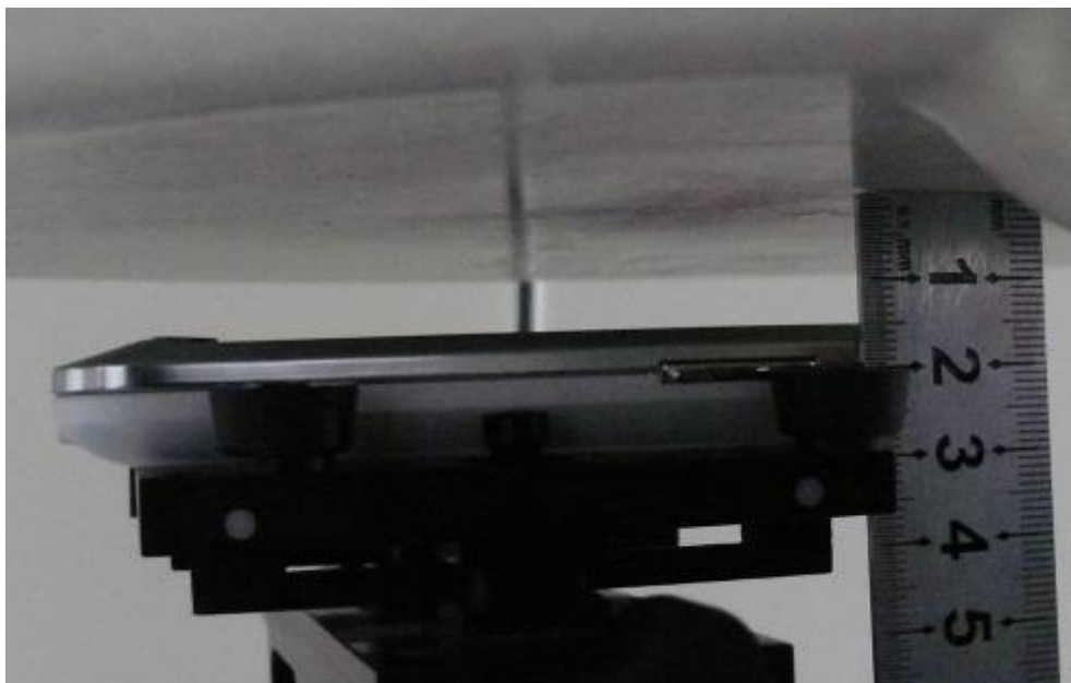
Picture 10: Body, The EUT display towards phantom, the distance from handset to the bottom of the Phantom is 15mm
