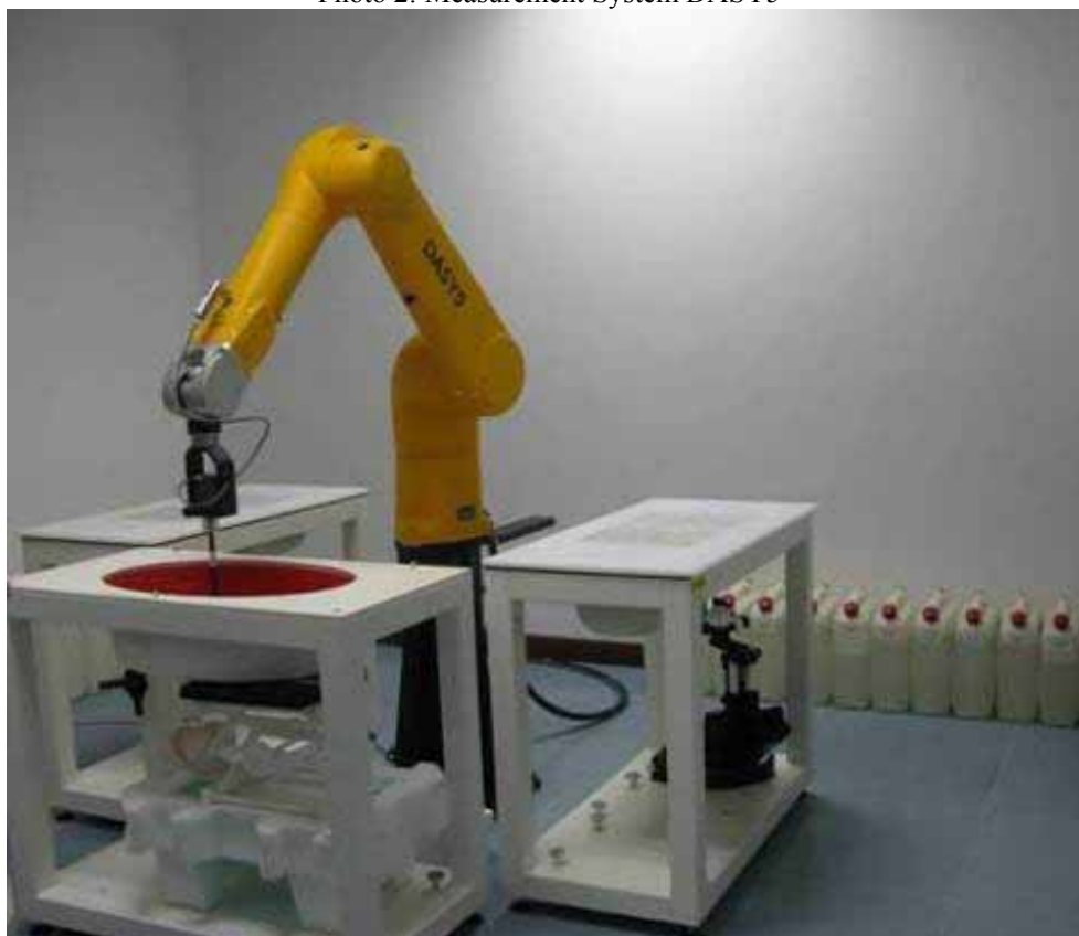
Photo 2: Measurement System DASY5
