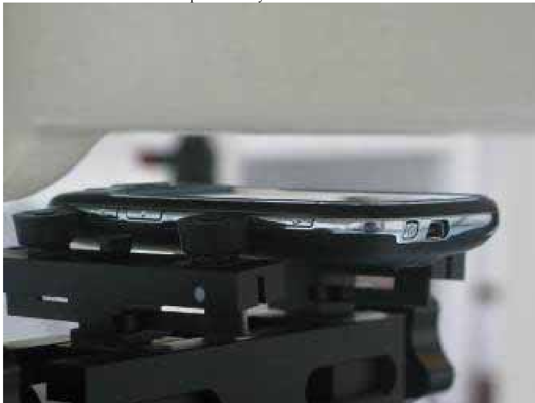
Photo 10: U7510 Test position body worn rear side with 15 mm distance
