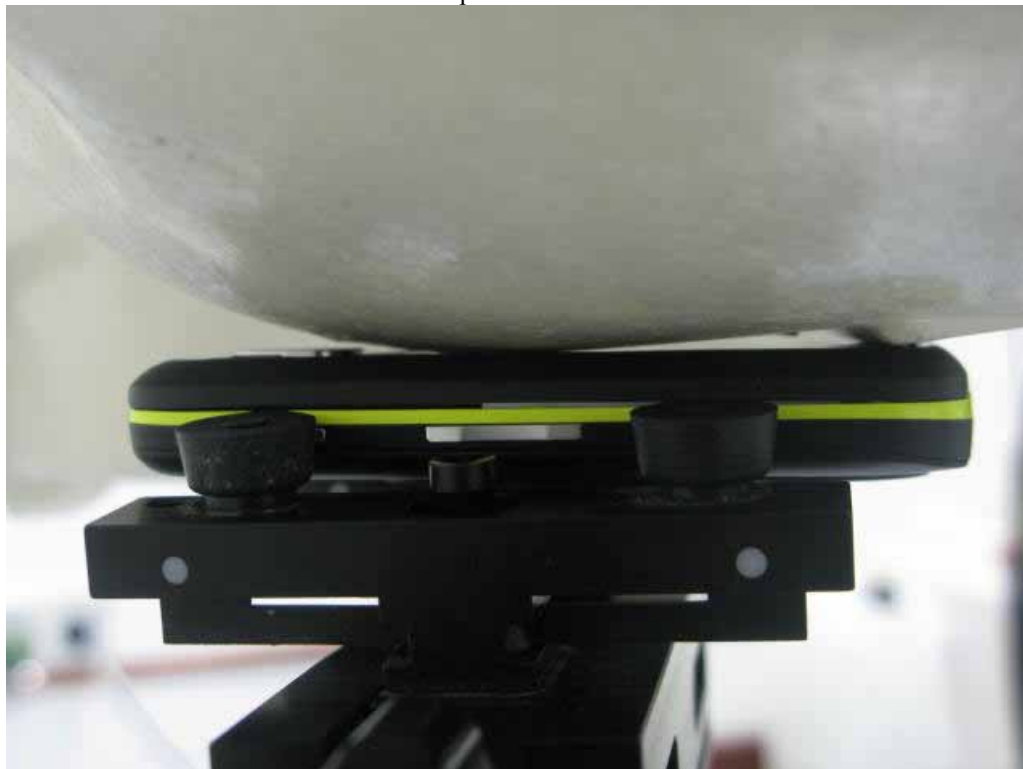
Photo 8: U3205 Test position left hand tilted 15°-Close
