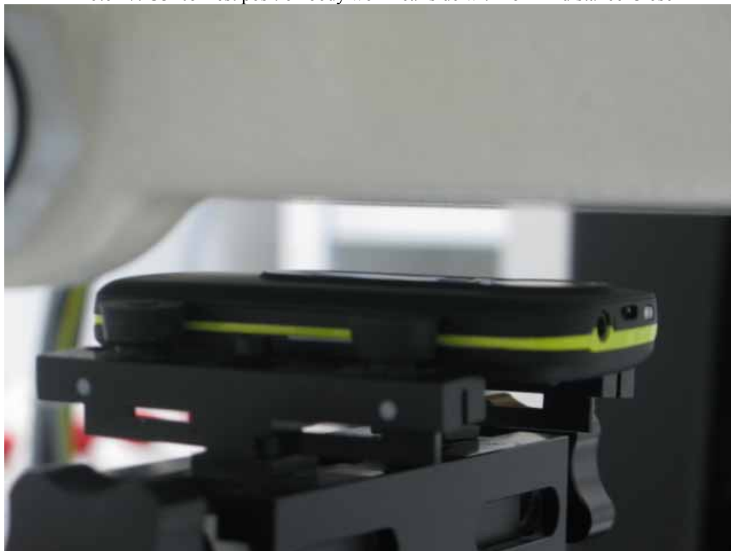
Photo 18: U3205 Test position body worn rear side with 15 mm distance-Open
