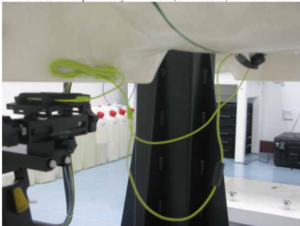
Photo 20: U3205 Test position body worn rear side (15 mm distance) with headset-Open
