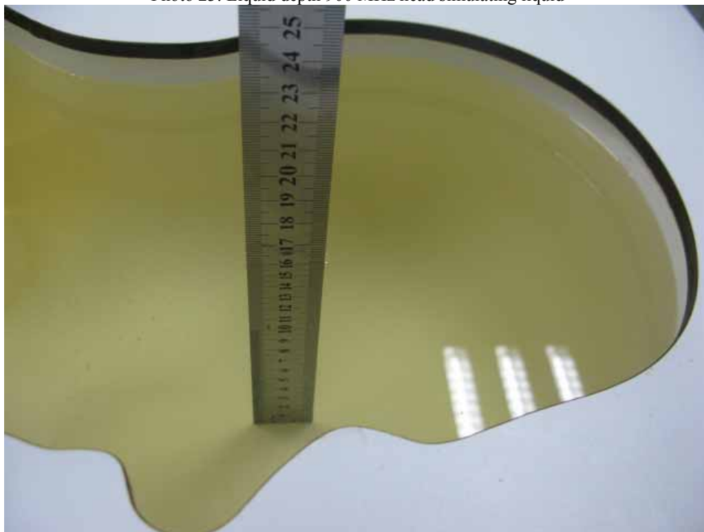
Photo 24: Liquid depth 900 MHz body simulating liquid
