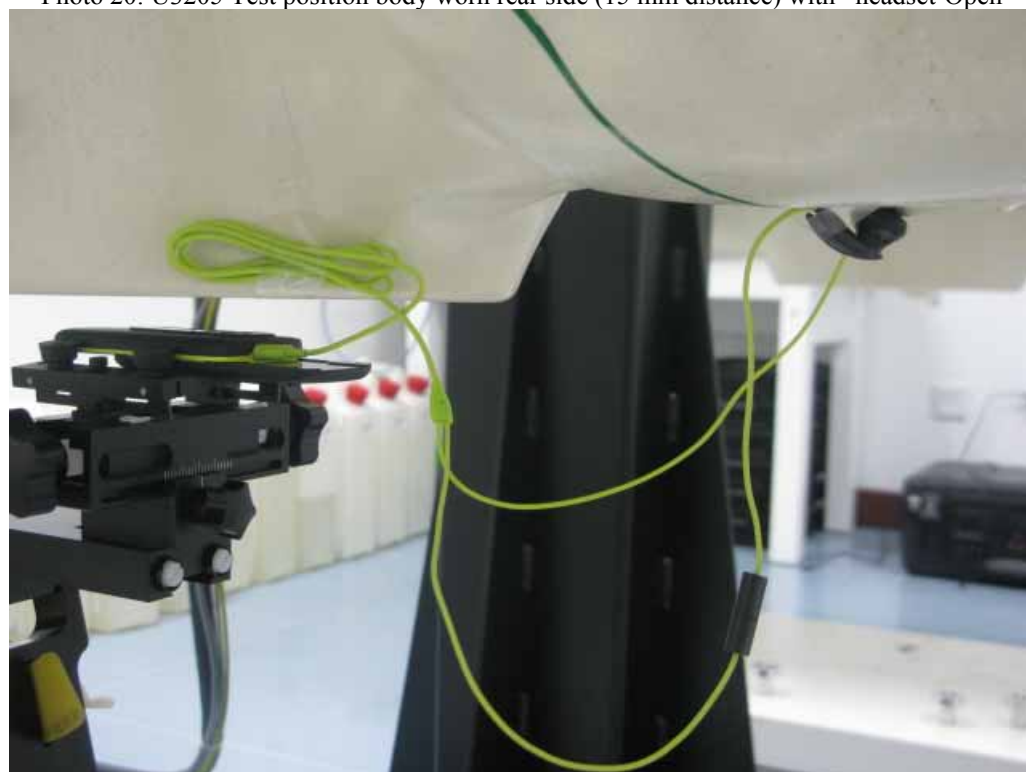
Photo 20: U3205 Test position body worn rear side (15 mm distance) with headset-Open
