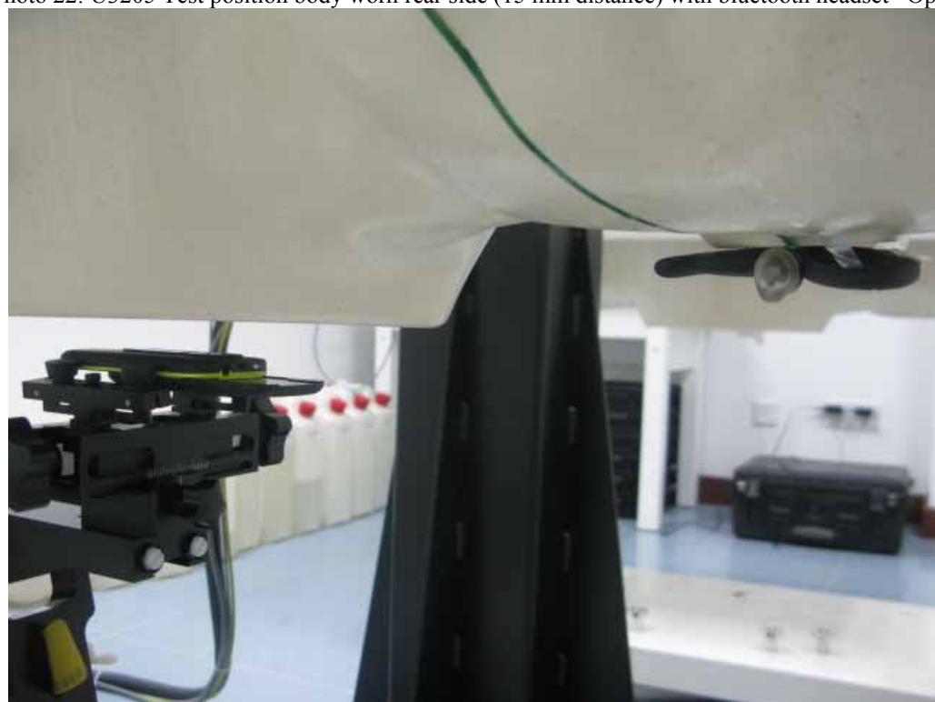
Photo 22: U3205 Test position body worn rear side (15 mm distance) with bluetooth headset –Open
