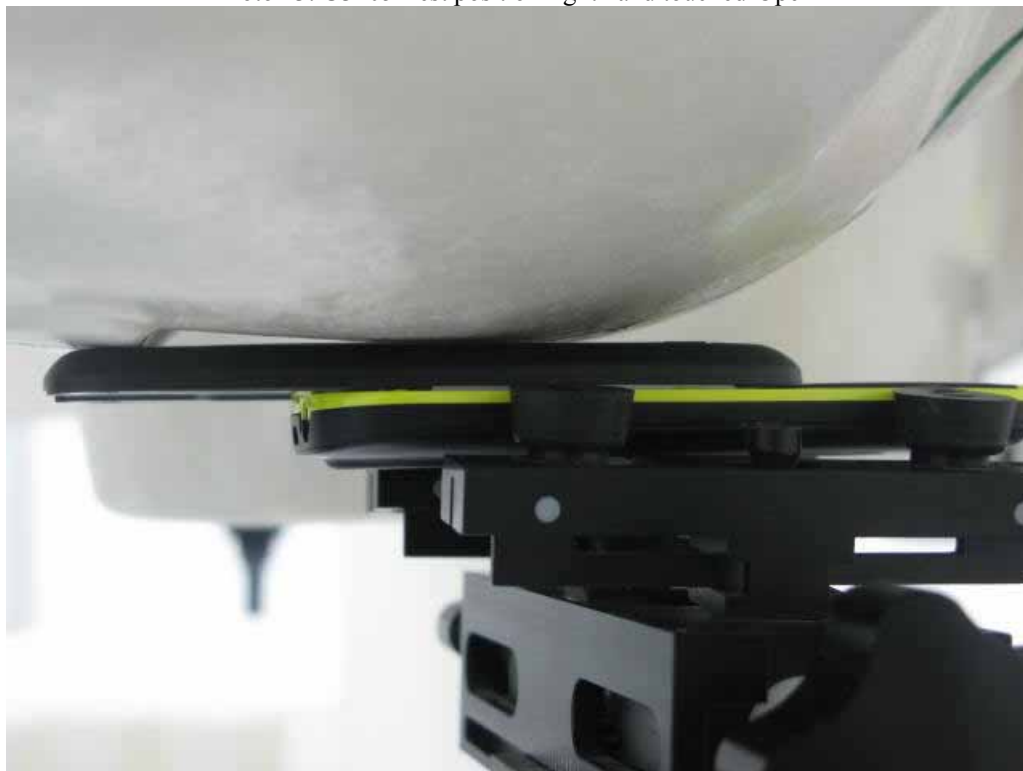
Photo 14: U3205 Test position right hand tilted 15° -Open
