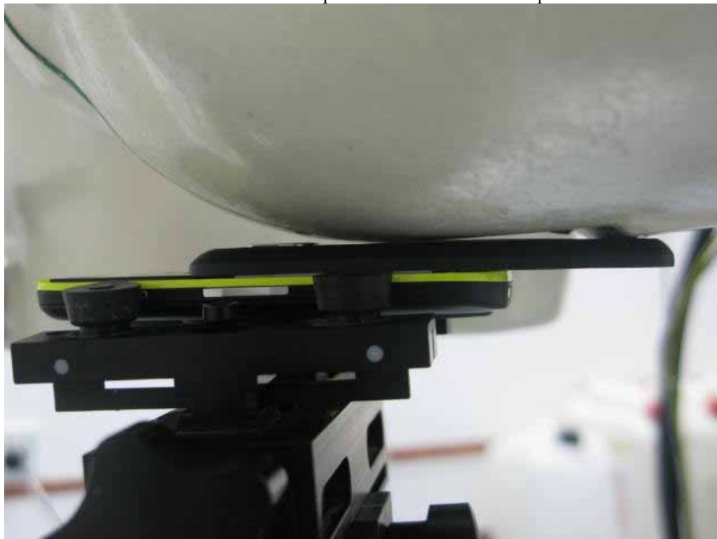
Photo 10: U3205 Test position left hand tilted 15°-Open
