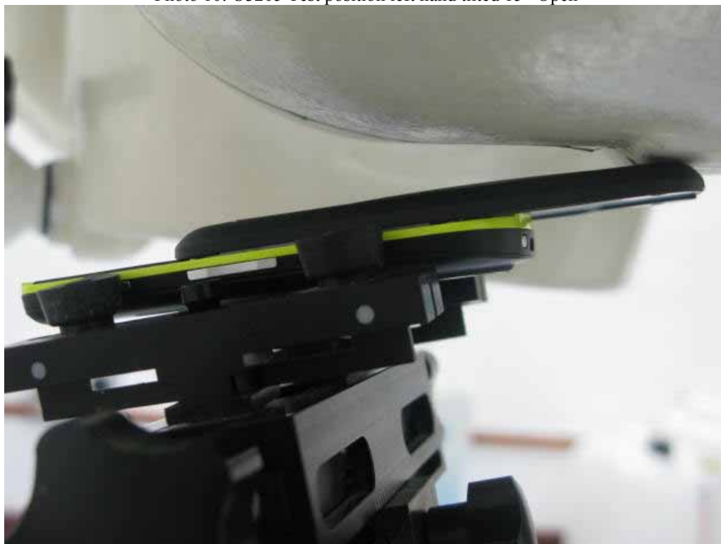
Photo 10: U3205 Test position left hand tilted 15°-Open
