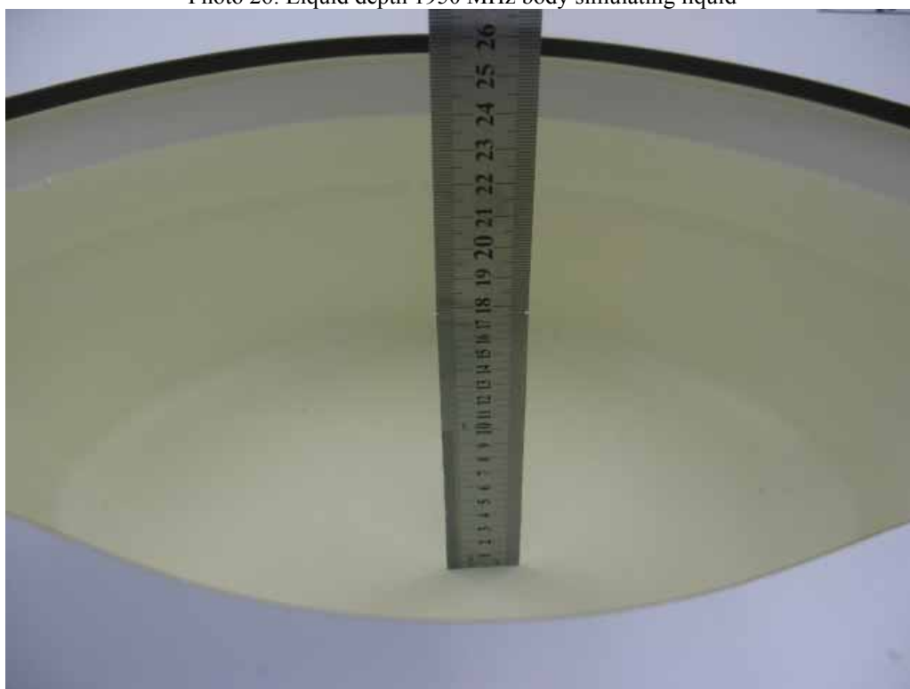
Photo 26: Liquid depth 1950 MHz body simulating liquid
