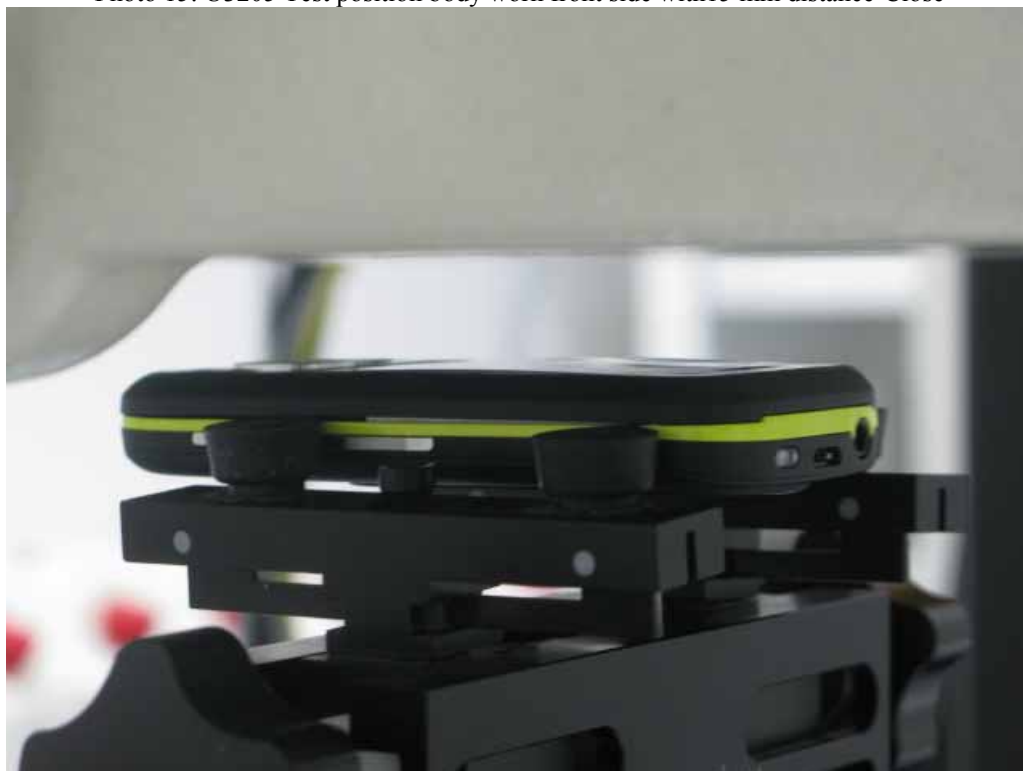
Photo 16: U3205 Test position body worn front side with15 mm distance-Open
