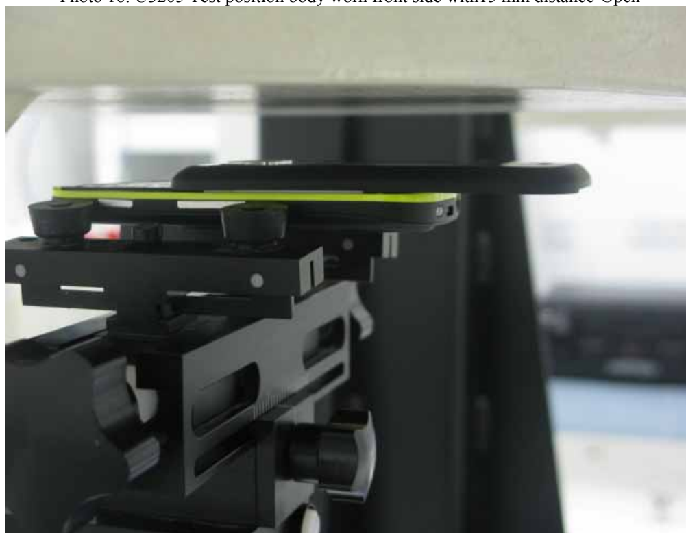
Photo 16: U3205 Test position body worn front side with15 mm distance-Open
