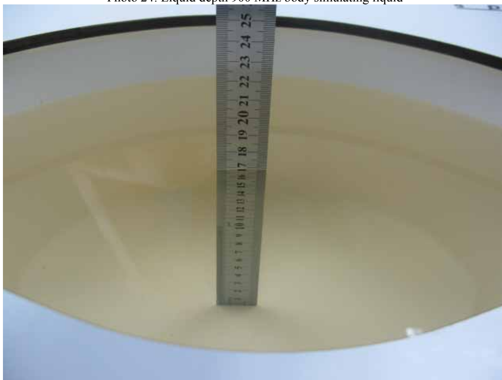
Photo 24: Liquid depth 900 MHz body simulating liquid
