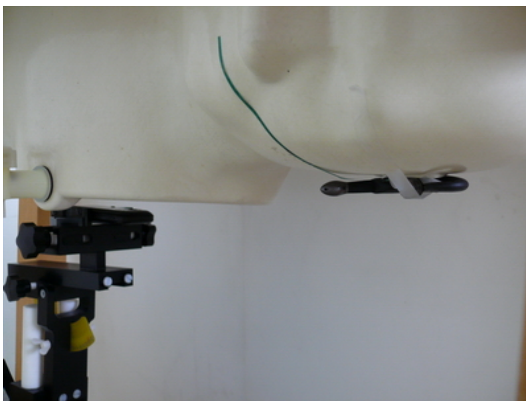
Picture 12: Body with the Bluetooth earphone, towards ground, the distance from handset to the bottom of the Phantom is 15mm)
