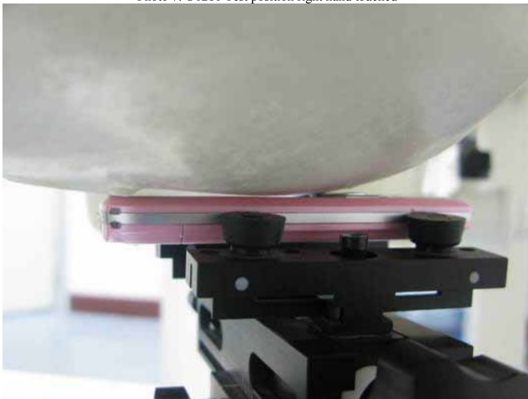
Photo 8: U1280 Test position right hand tilted 15°
