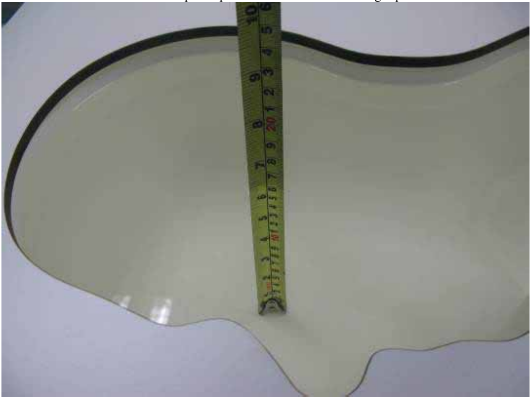
Photo 14: Liquid depth 1950 MHz body simulating liquid
