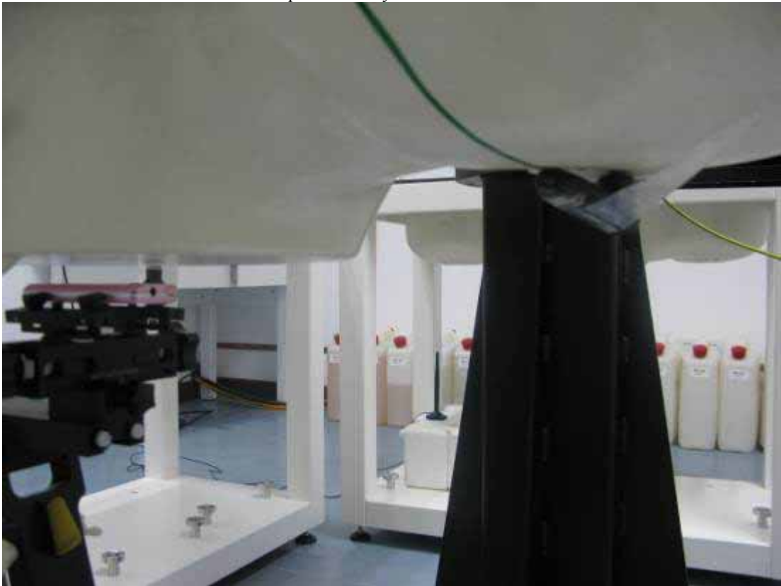
Photo 12: U1280 Test position body worn rear side with 15 mm distance
