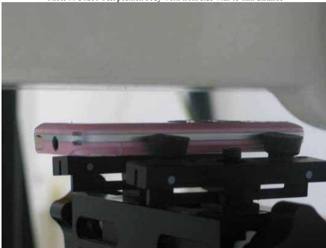
Photo 10: U1280 Test position body worn rear side with 15 mm distance
