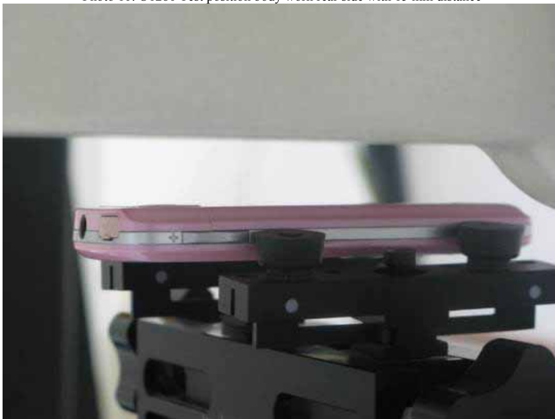
Photo 10: U1280 Test position body worn rear side with 15 mm distance
