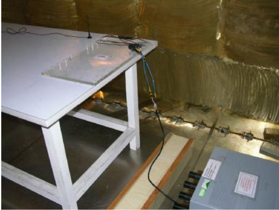
Conducted Emissions of AC Power Port
