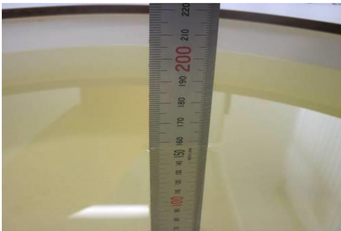
Picture 7-4: Liquid depth in the Flat Phantom (1800MHz)
