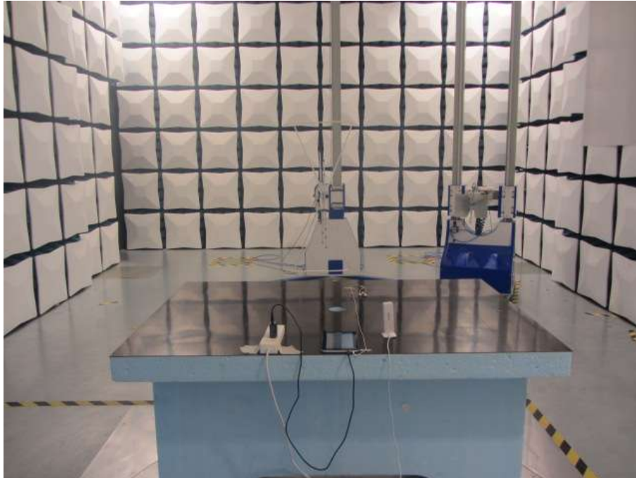
Radiated Spurious Emission (below 1GHz)
