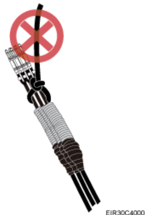
Figure 7-8 Incorrect binding method
