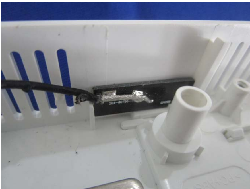
EUT – BT Antenna View
