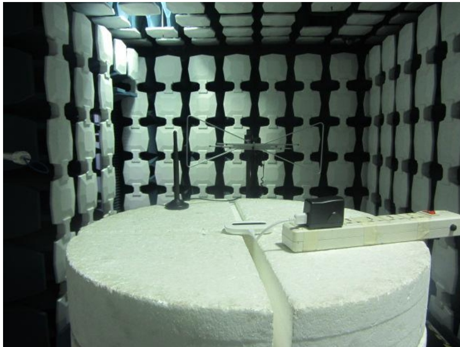
Radiated Spurious Emission (below 3GHz)
