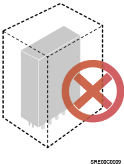
Figure 9-1 Inappropriately installed pRRU
