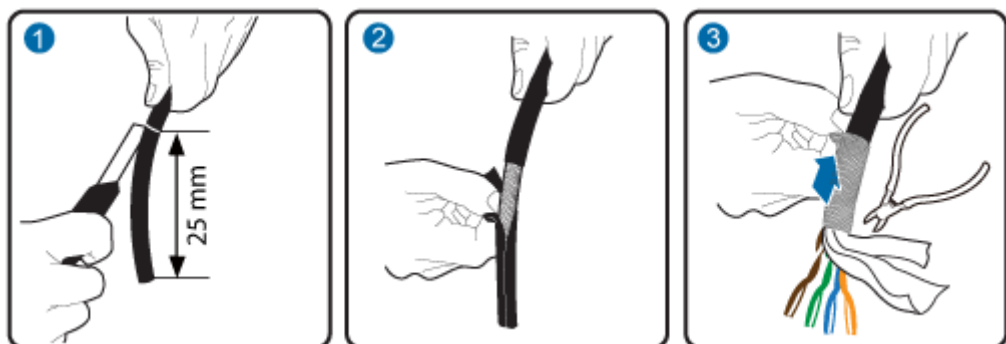
Figure 15-2 Removing the jacket of an Ethernet cable
