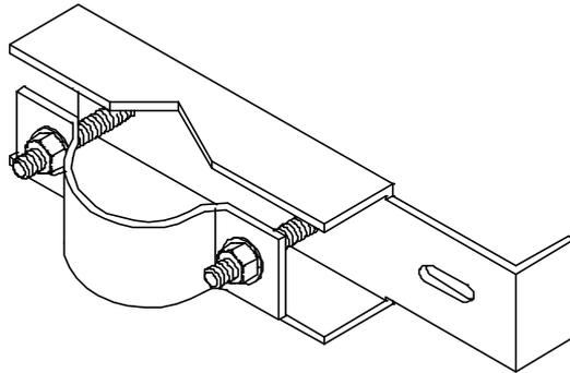
Figure 3-2 Omni antenna fixing clip (1)
