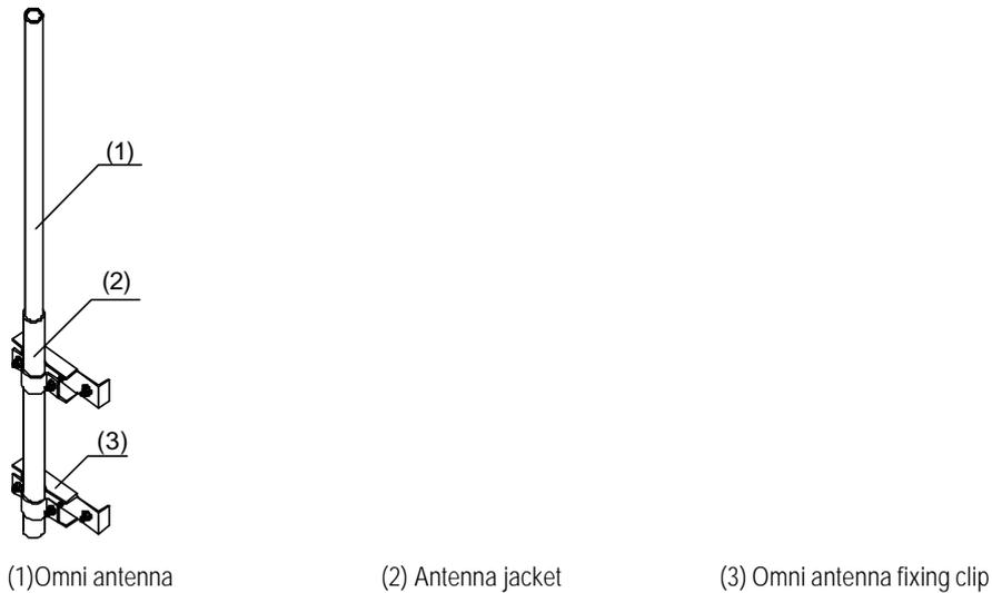
**Figure 3-4** Fixing omni antenna
