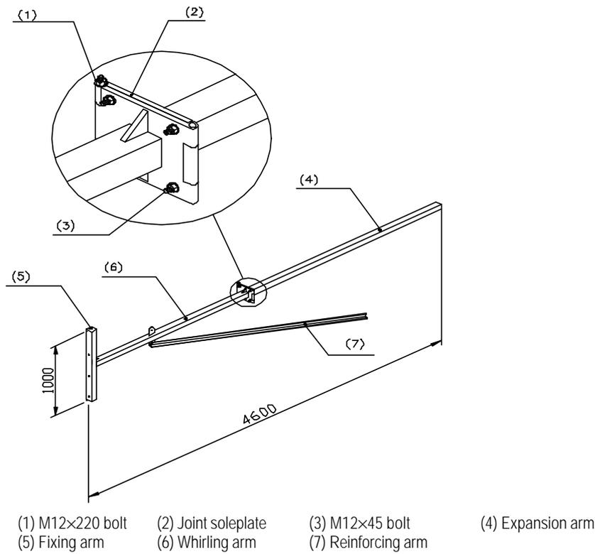
Figure 3-12 Structure of antenna support installed on tower
