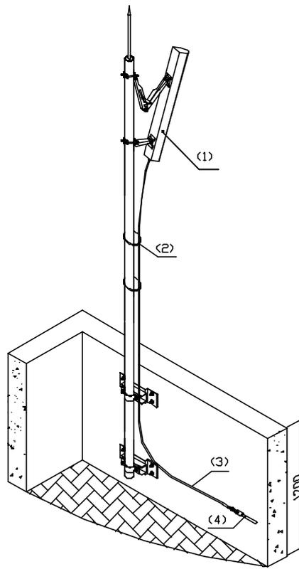
(1) Antenna      (2) Cable tie      (3) Jumper      (4) Feeder
