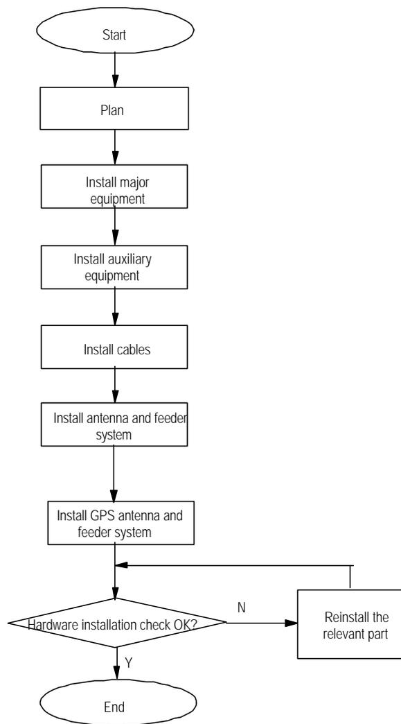
Figure 2-2 Hardware installation flow
