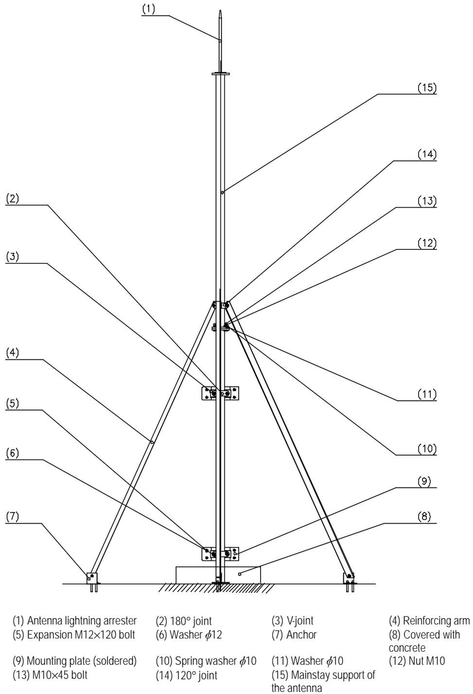
Figure 3-15 Structure of antenna support installed on building-top
