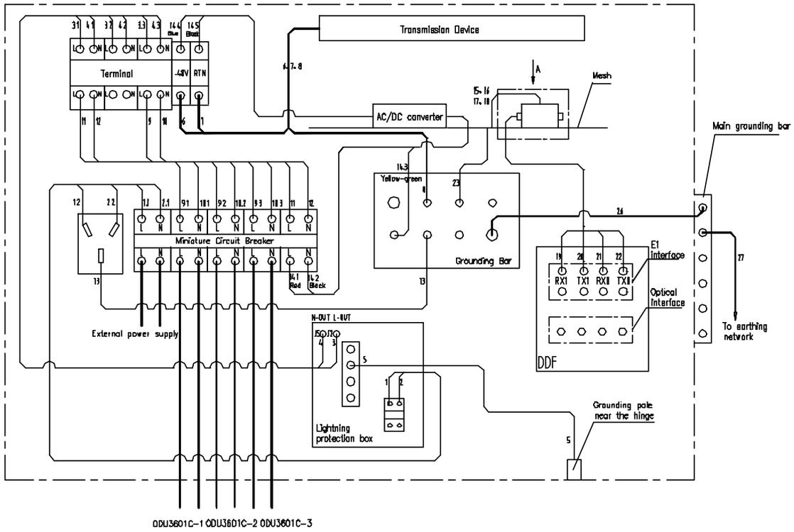
Figure 2-52 Cable distribution of IAFB networking (without UPS)
