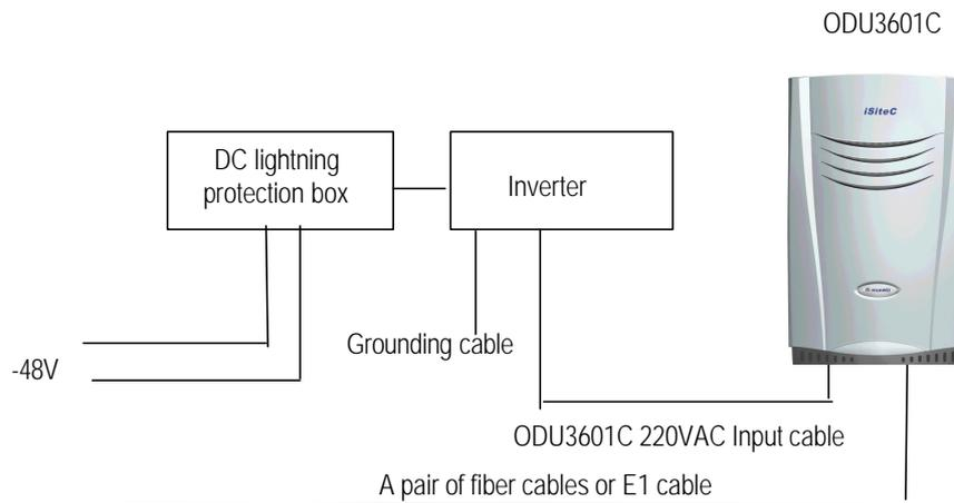
**Figure 2-61** Inverter networking
