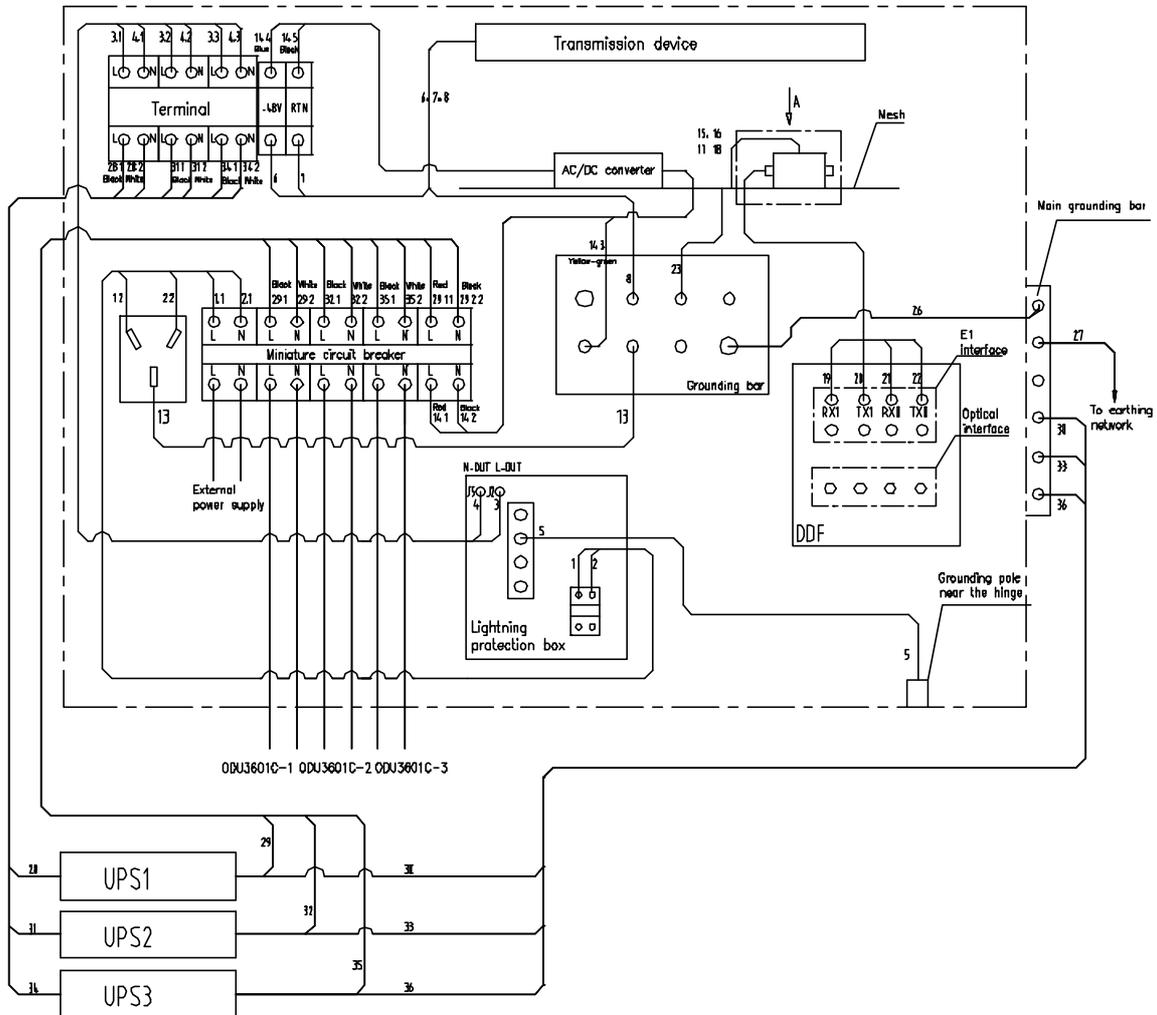
Figure 2-59 Cable distribution in IAFB networking (3 ODU3601Cs with UPS)
