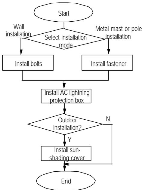
**Figure 2-34** Installation flow of AC lightning protection box
