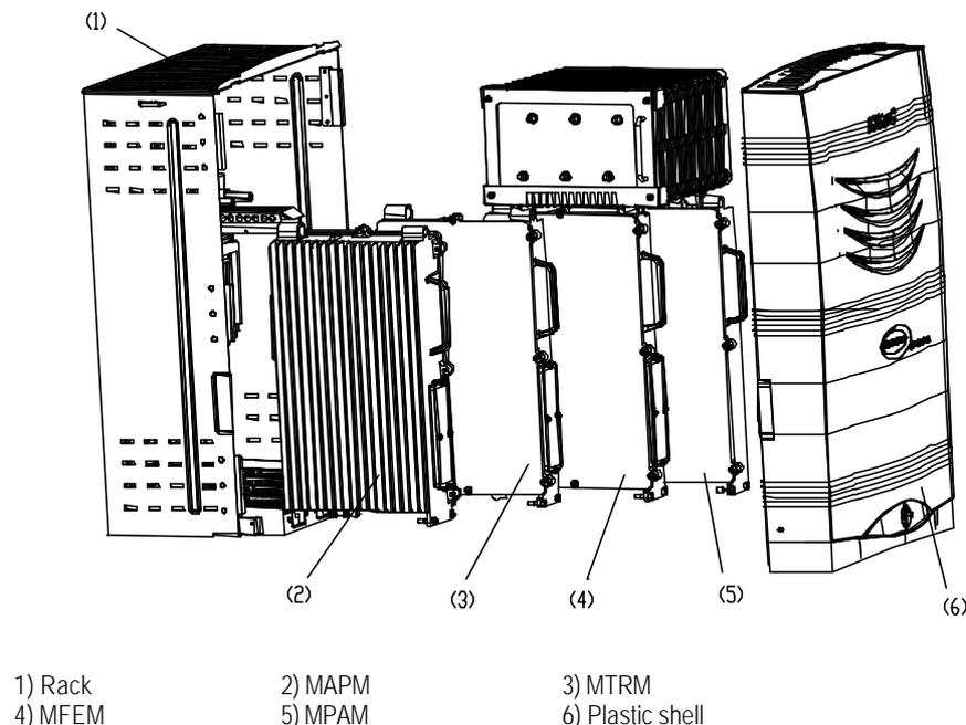
Figure 2-1 ODU3601C structure
