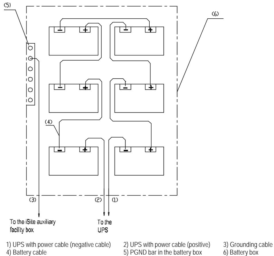
**Figure 2-44** Connecting UPS to the IABB
