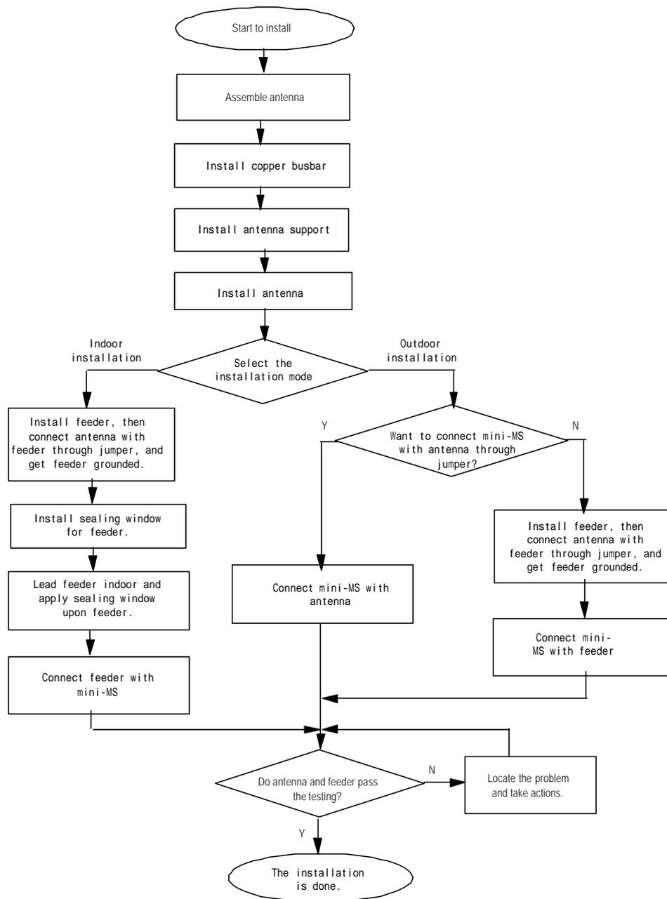
Figure 3-1 Installation flow of antenna and feeder system
