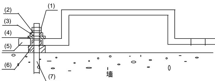
(1) Nut M12                      (2) Spring washer  $\phi 12$                       (3) Large plain washer                      (4) Insulation washer 1
