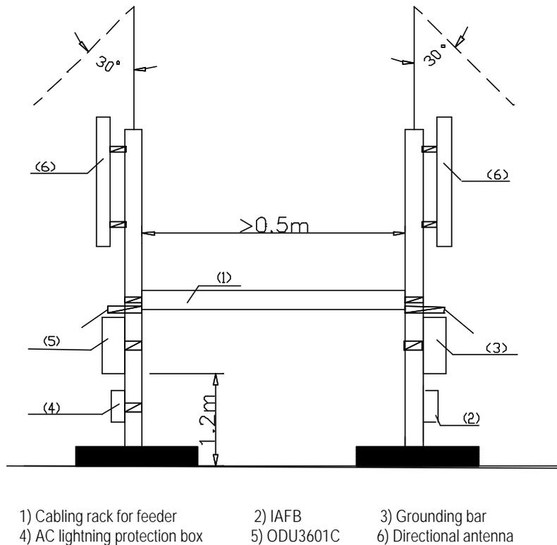
Figure 2-7 Directional ODU3601C installation on metal masts
