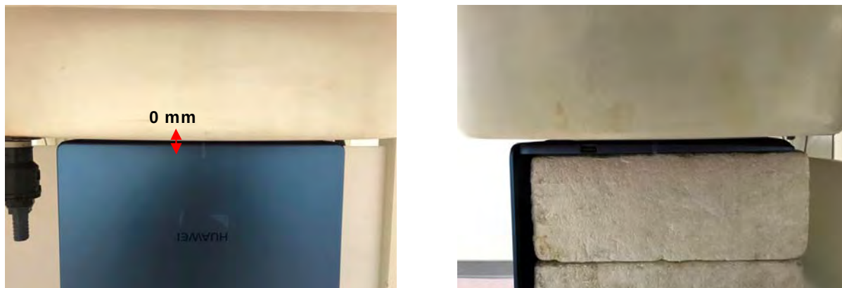
Fig.3 EUT Bottom side to flat phantom
