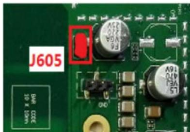
Figure 4 Jump Wire Configuration
