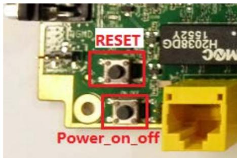
Figure 6 Keys to Turning-on and Reset
