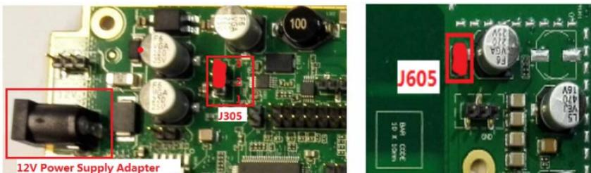
**Figure 2 12V Power Supply on the DVK**
