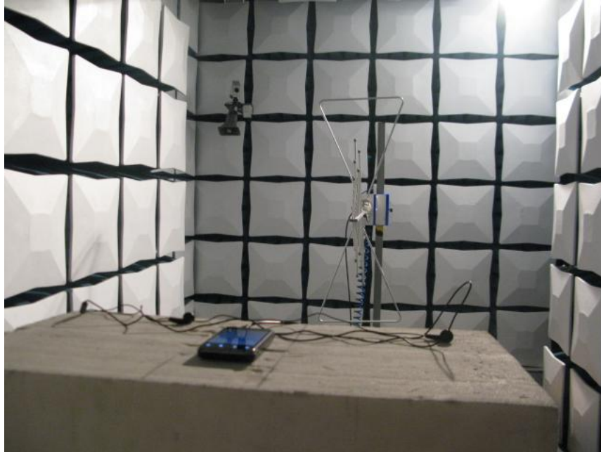
Radiated Spurious Emission (below 3GHz)
