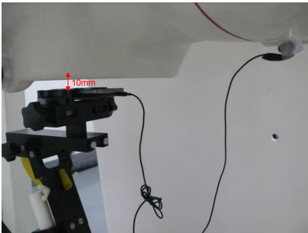
Picture 16: Body with Earphone, The EUT display towards phantom, the distance from handset to the bottom of the Phantom is 10mm
