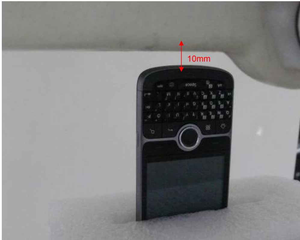
Picture 19: Bottom edge, the distance from handset to the bottom of the Phantom is 10mm
