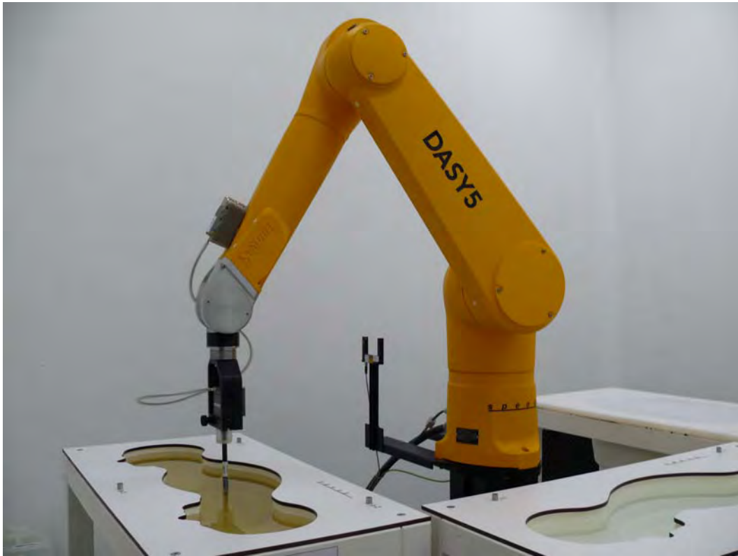
Picture 1: Specific Absorption Rate Test Layout
