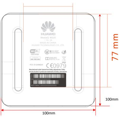
Refer the picture above, the product size is  $100 \times 100 \text{mm}$  and the maximum size of the label area is only  $52 \times 77 \text{mm}$ . Due to the target market of this product to several countries and lots of certification marks needed to adding on the product, so it's no place to adding the FCC statement and we put this statement in the user manual instead of on the product.
