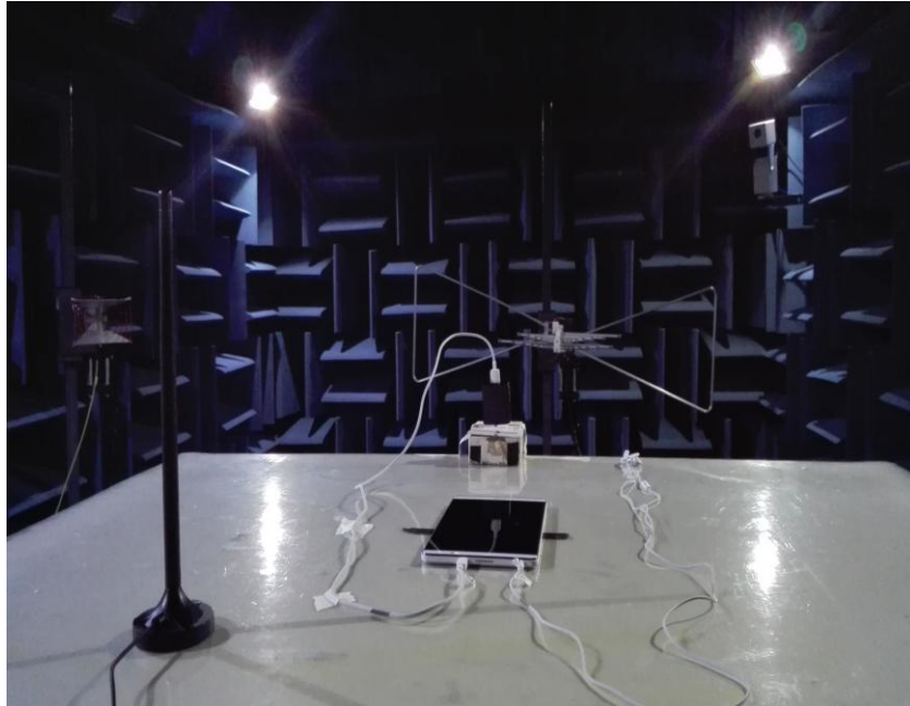
Radiated Spurious Emission (1GHz to18GHz)
