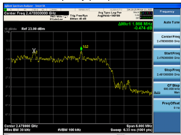
BT 2MHz \pi/4 -DQPSK(4Mbps) CH37, Carrier frequency (MHz): 2478
