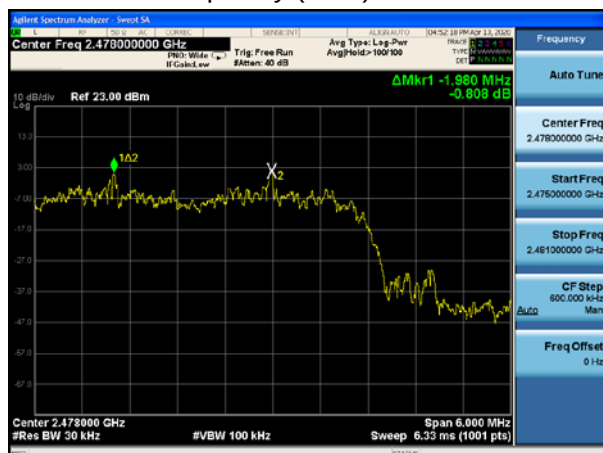
BT 2MHz 8DPSK(6Mbps) CH37, Carrier frequency (MHz): 2478
