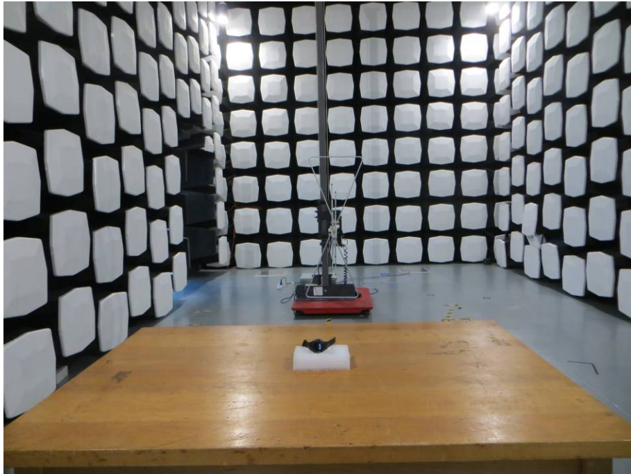
3. Radiated Emissions (Part 15C) 30M-1GHz)
