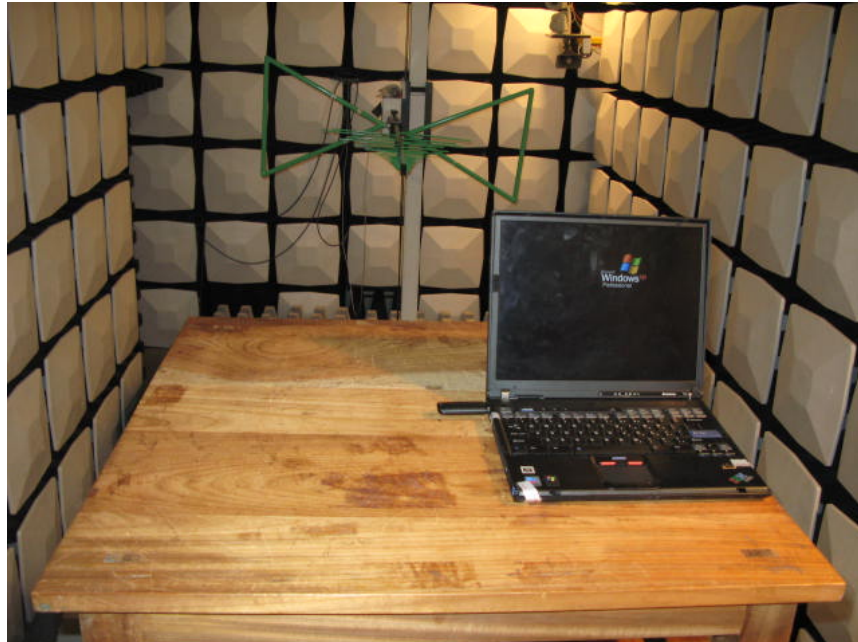
Radiated Spurious Emission (below 2GHz)
