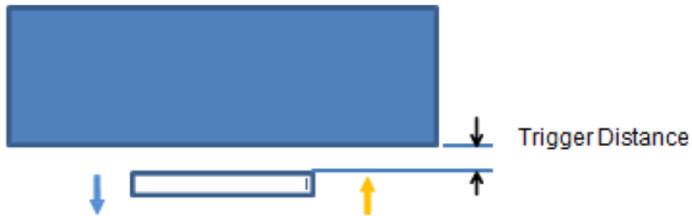
Picture: Proximity sensor triggering distances assessment (Front/Back side)
