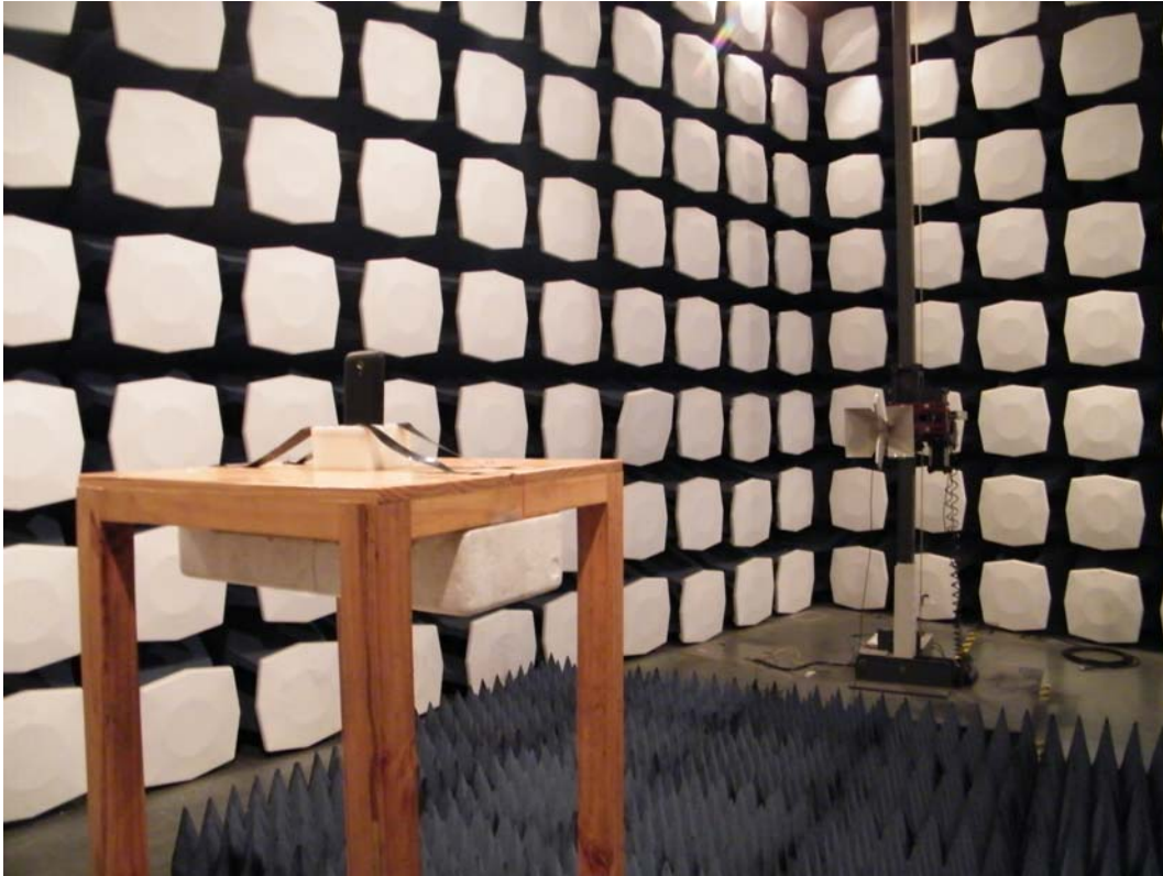
Picture 2: Radiated Spurious Emissions Test setup
