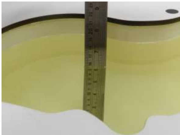
Fig 10.1 Photo of Liquid Height for Head SAR
