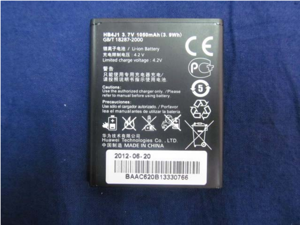
(10) EUT Photo (Battery #1)
