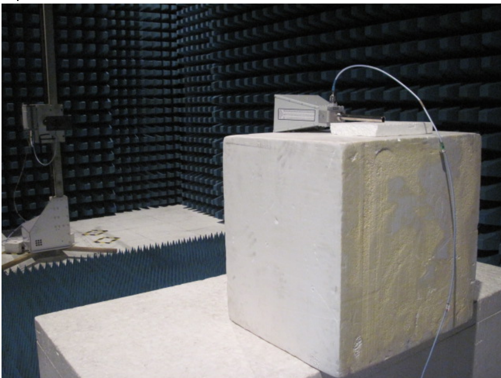
Description: Substitution Antenna for EIRP Test
