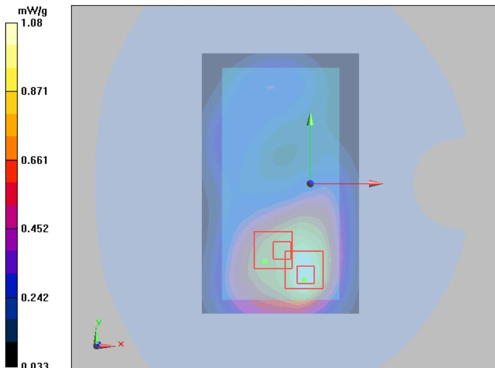
Figure 63 Body, Front Side, UMTS Band II Channel 9400
