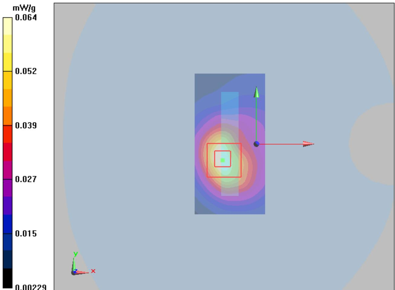
Figure 28 Body, Bottom Edge, GSM 850 GPRS (TX slot) Channel 190
