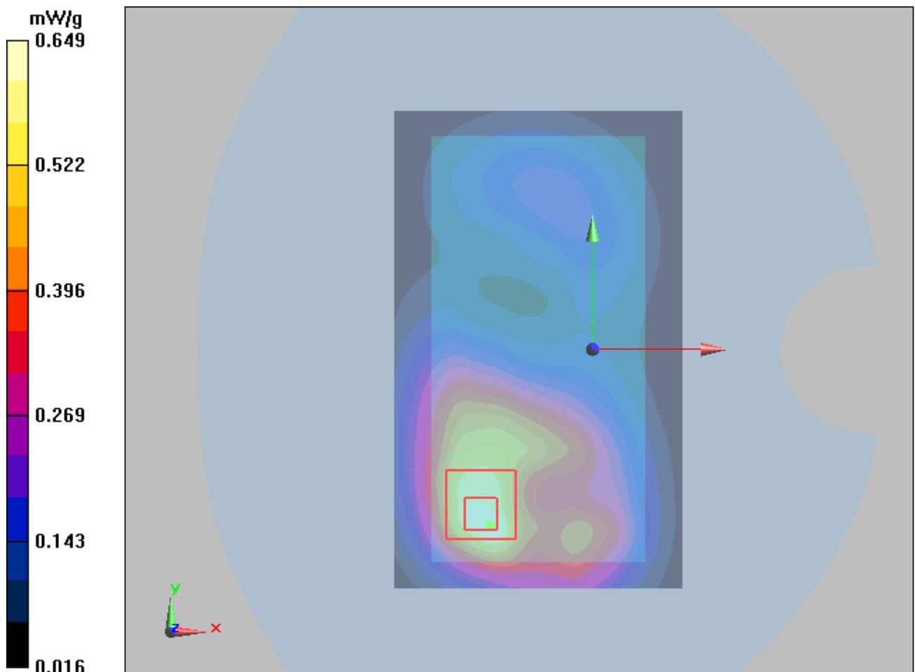
Figure 46 Body, back side, GSM 1900 EGPRS (1Txslot) Channel 661
