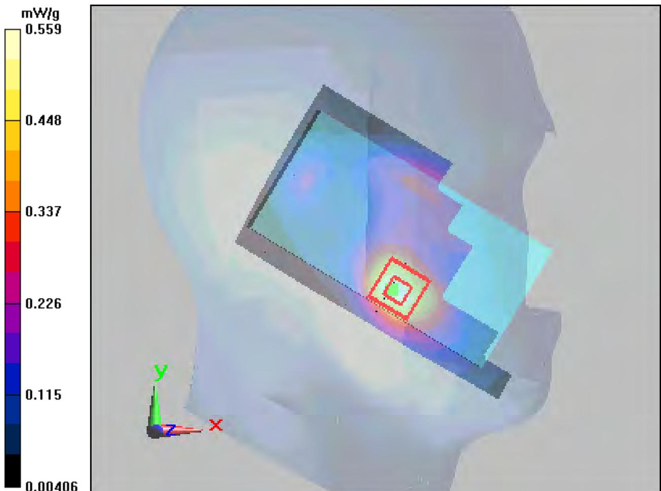
Figure 49 Left Hand Touch Cheek UMTS Band II Channel 9538
