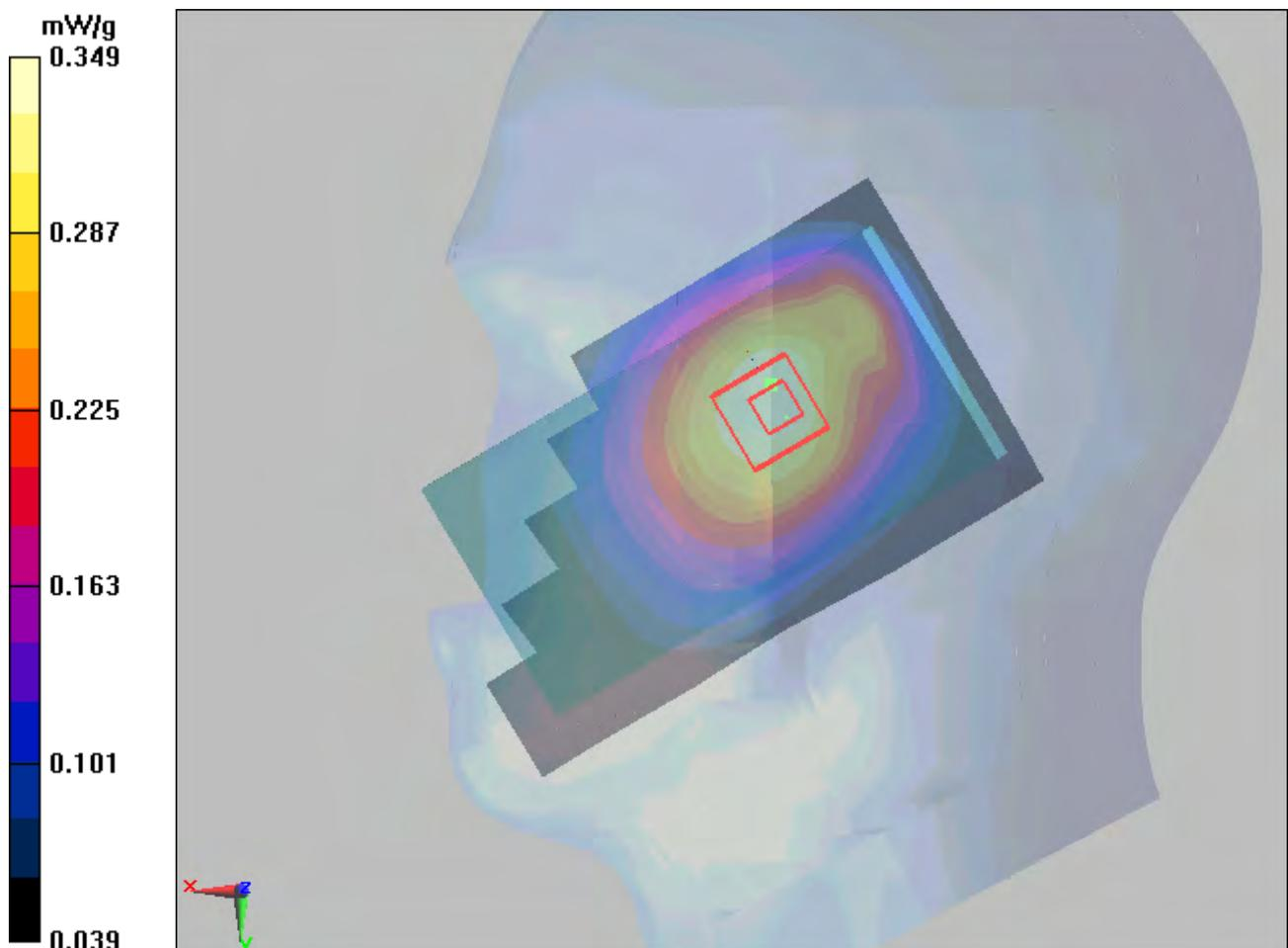
Figure 16 Right Hand Tilt 15° GSM 850 Channel 190
