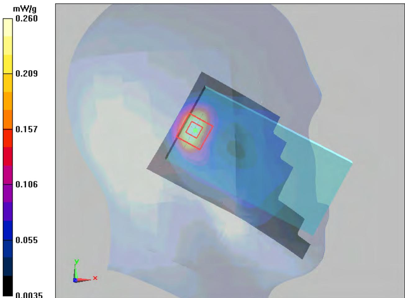
Figure 35 Left Hand Tilt 15° GSM 1900 Channel 661
