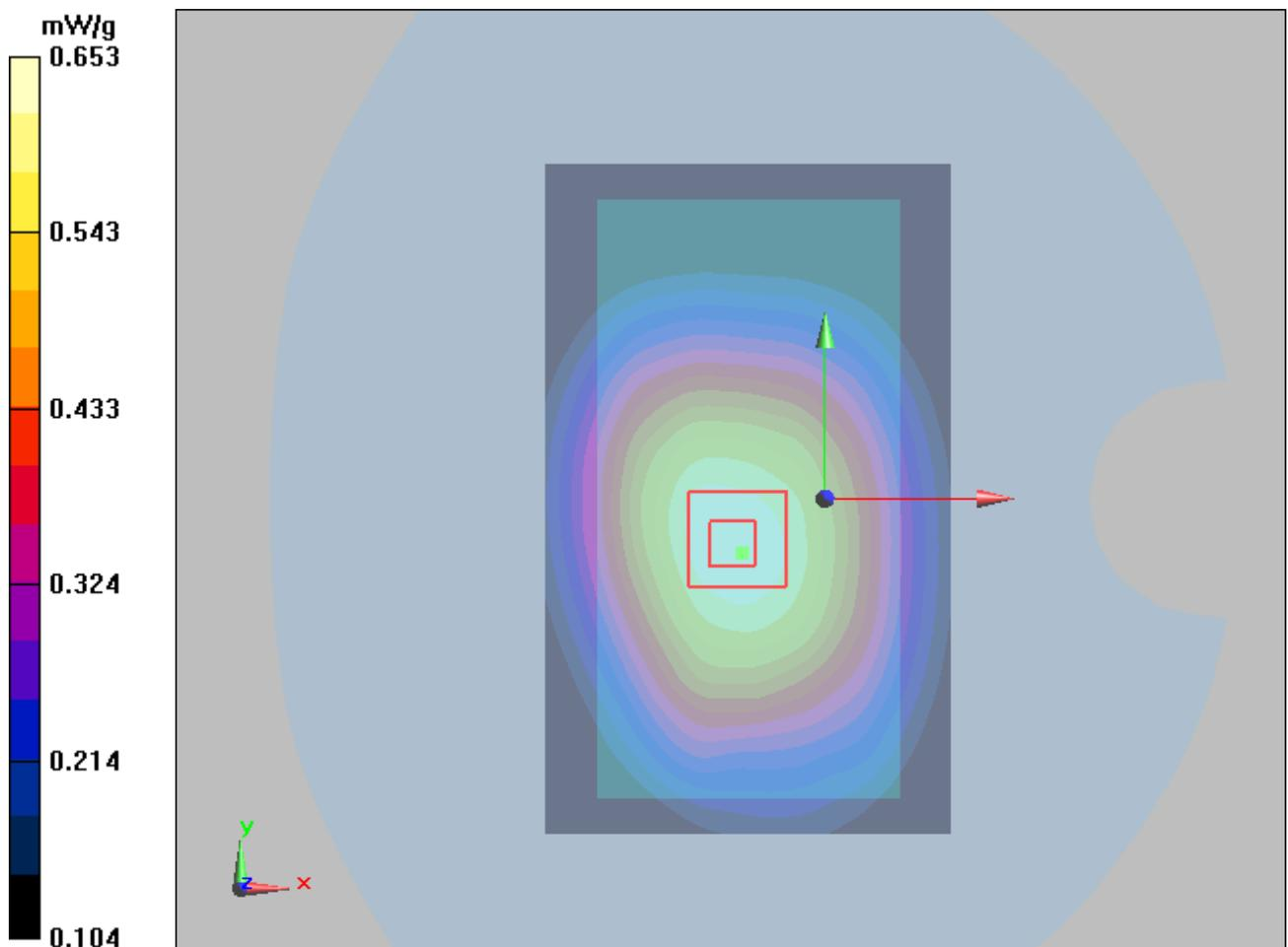
Figure 25 Body, Front Side, GSM 850 GPRS (1Txslot) Channel 190
