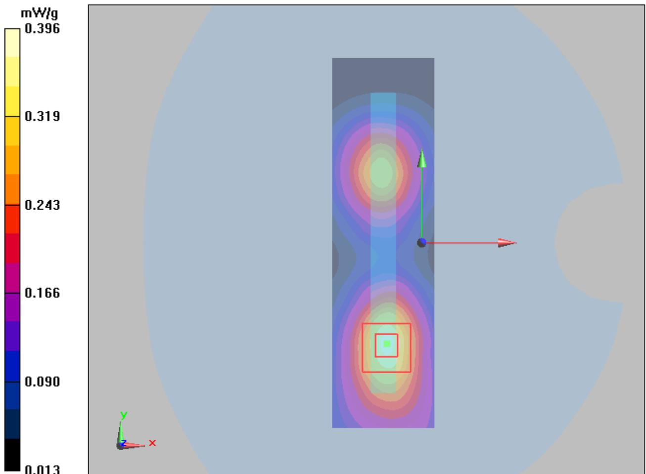
Figure 65 Body, Left Edge, UMTS Band II Channel 9400
