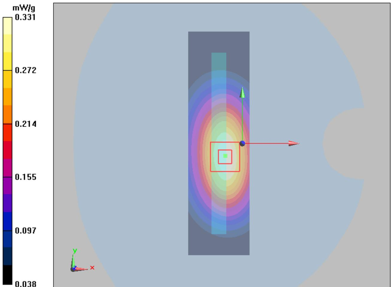
Figure 27 Body, Right Edge, GSM 850 GPRS (1Txslot) Channel 190
