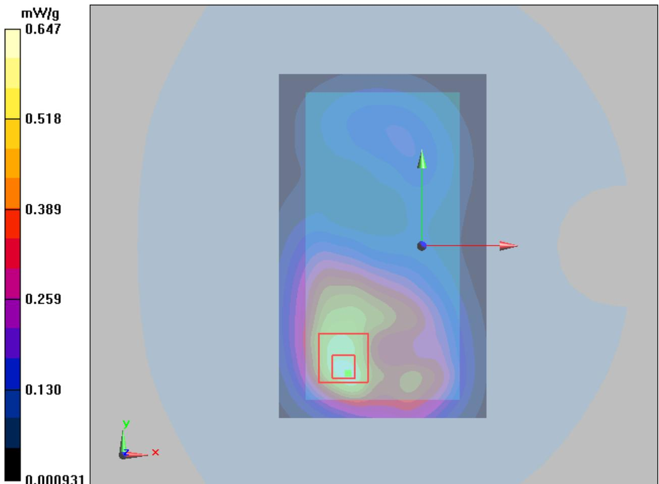
Figure 40 Body, Back Side, GSM 1900 GPRS (1Txslot) Channel 661
