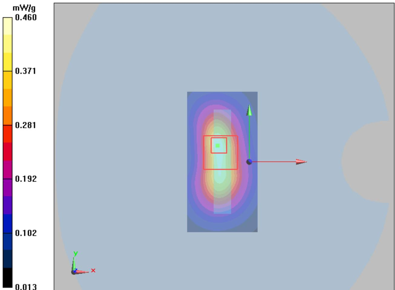
Figure 45 Body, Bottom Edge, GSM 1900 GPRS (1Txslot) Channel 661
