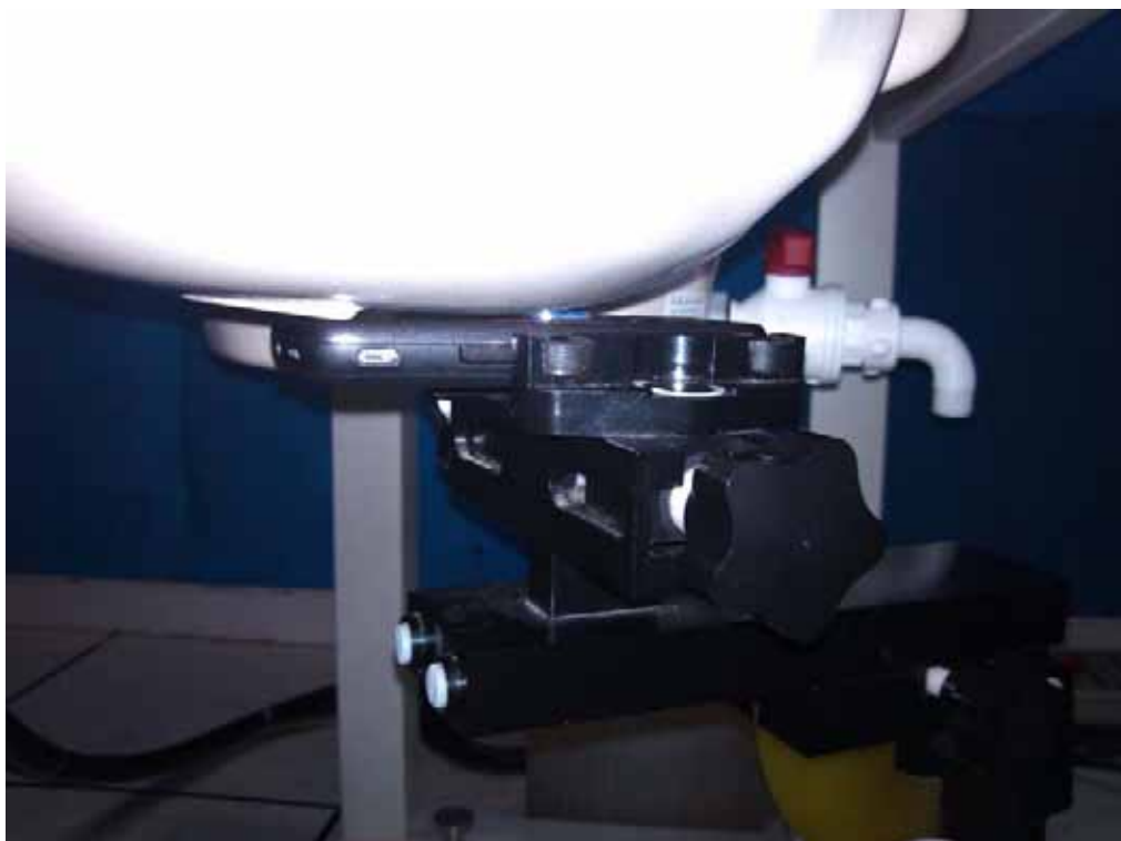
Picture 16-4: Right Hand Touch Cheek Position
