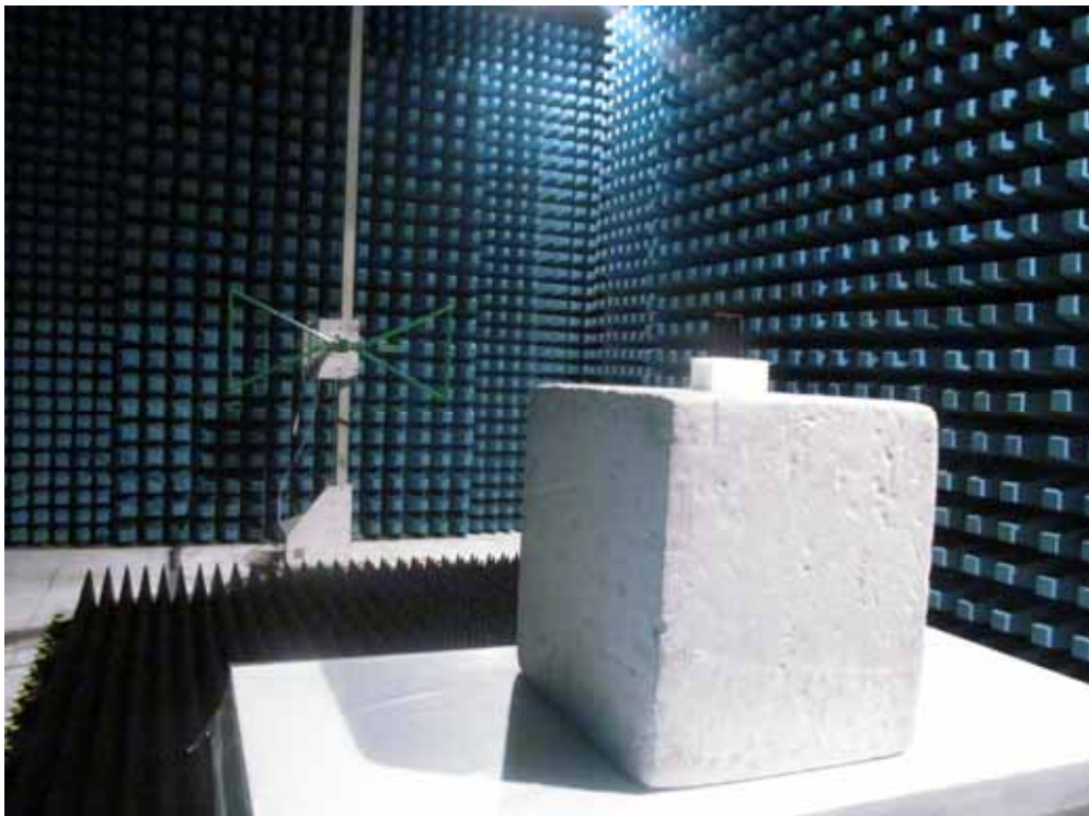
Description: ERP Test Setup
